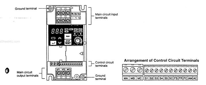
Note: This illustration shows the terminal block with the front cover removed.
