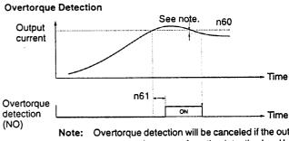
Overtorque detection will be canceled if the output current decreases from the detection level by approximately 5% of the Inverter rated current.
