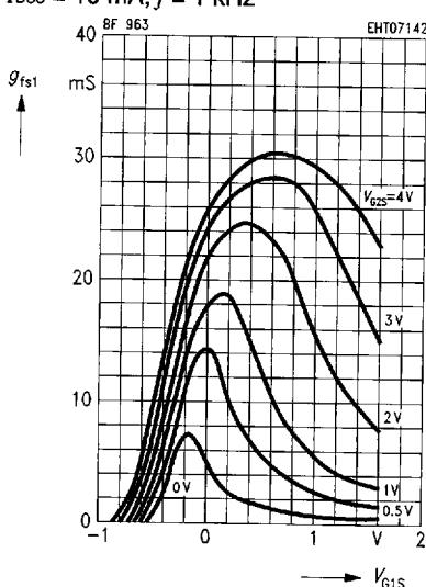
Gate 1 forward transconductance  $g_{fs1} = f(V_{G2S})$  $V_{DS} = 15 \text{ V}$  $I_{DSS} = 10 \text{ mA}, f = 1 \text{ kHz}$
