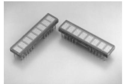
adjusting the display intensity and power consumption. The HDSP-213X is designed for standard microprocessor interface techniques. The display and special features are accessed through a bidirectional eight-bit data bus. These features make the HDSP-213X ideally suited for applications where a hermetic, low power alphanumeric display is required.
