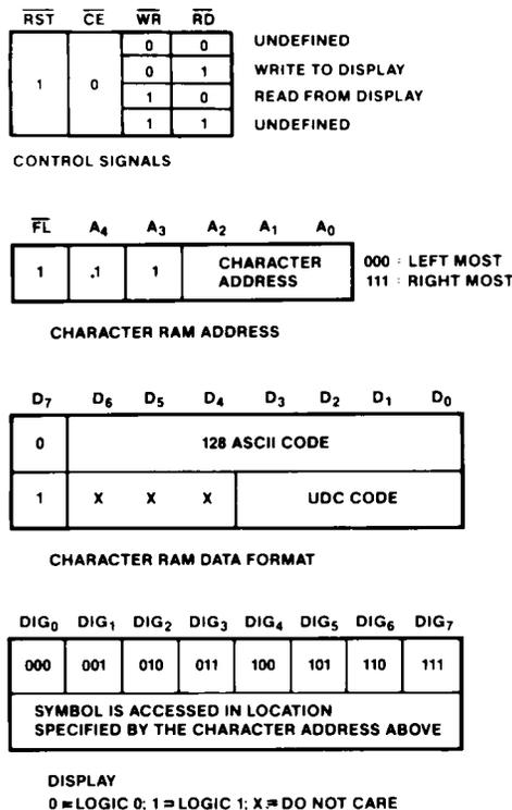
Figure 2. Logic Levels to Access the Character RAM.
