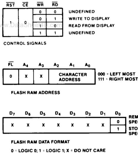
Figure 5. Logic Levels to Access the Flash RAM.
