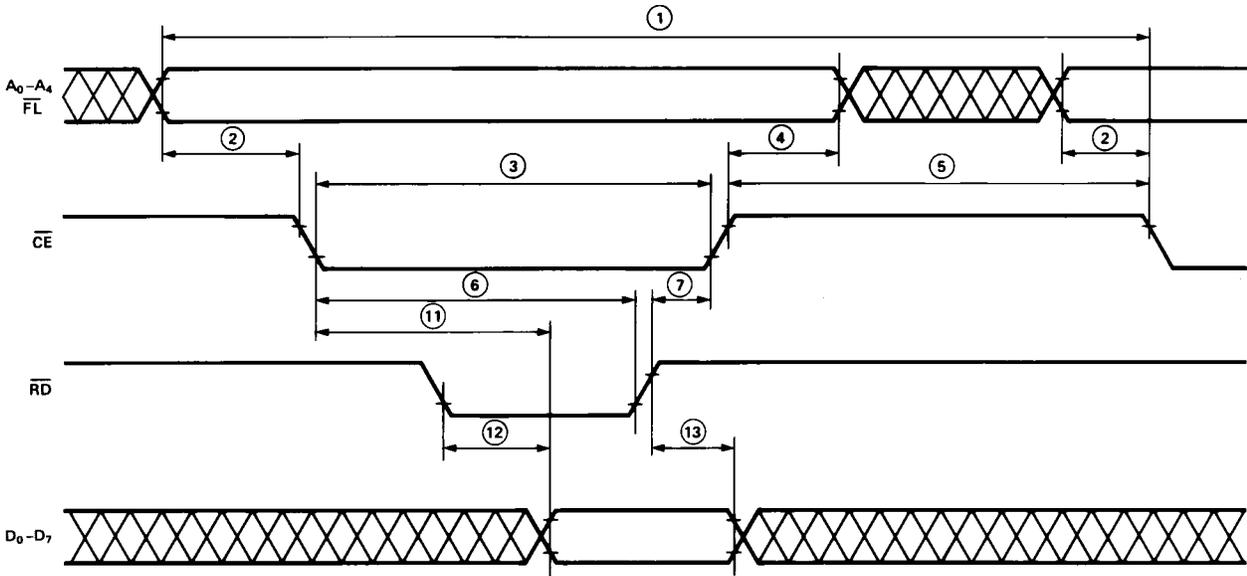
INPUT PULSE LEVELS: 0.6 V TO 2.4 V
