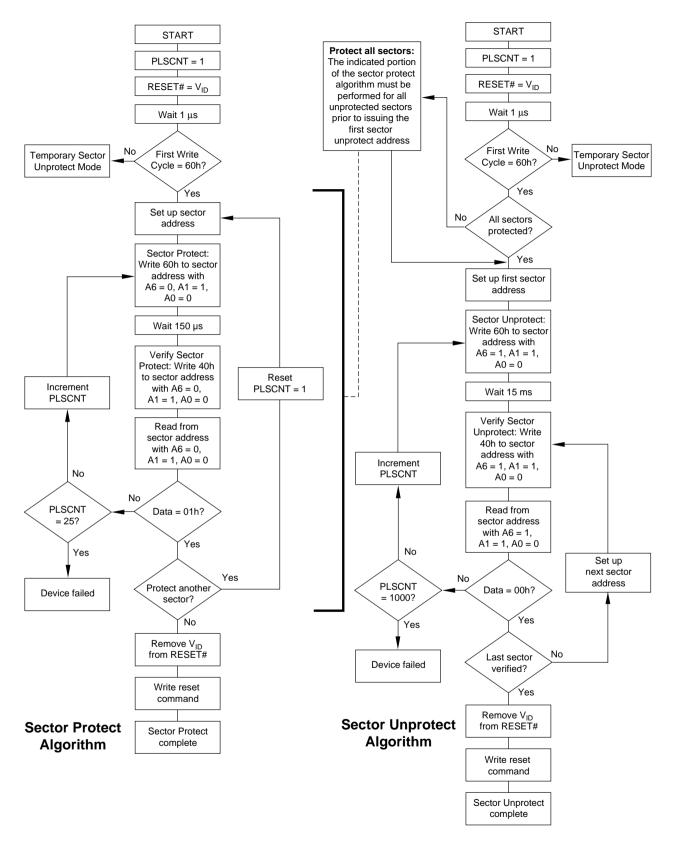
Figure 2. In-System Sector Protect/Unprotect Algorithms
