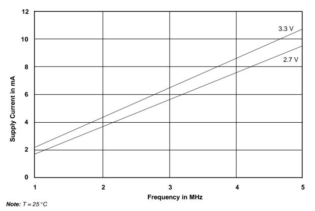
Figure 10. Typical I<sub>CC1</sub> vs. Frequency
