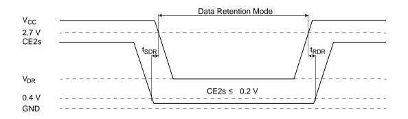
Figure 34. CE2s Controlled Data Retention Mode
