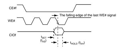
**Note:** Refer to the Erase/Program Operations table for  $t_{AS}$  and  $t_{AH}$  specifications.
