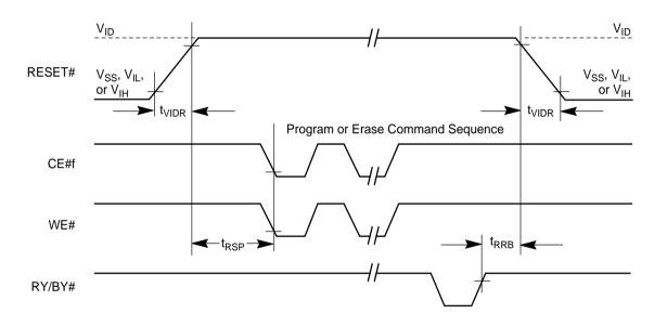
Figure 25. Temporary Sector Unprotect Timing Diagram
