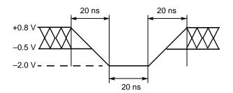
Figure 7. Maximum Negative Overshoot Waveform
