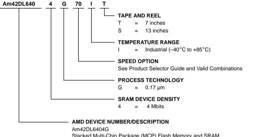
Stacked Multi-Chip Package (MCP) Flash Memory and SRAM Am29DL640G 64 Megabit (8 M x 8-Bit/4 M x 16-Bit) CMOS 3.0 Volt-only, Simultaneous Operation Flash Memory and 4 Mbit (256 K x 16-Bit) Static RAM
