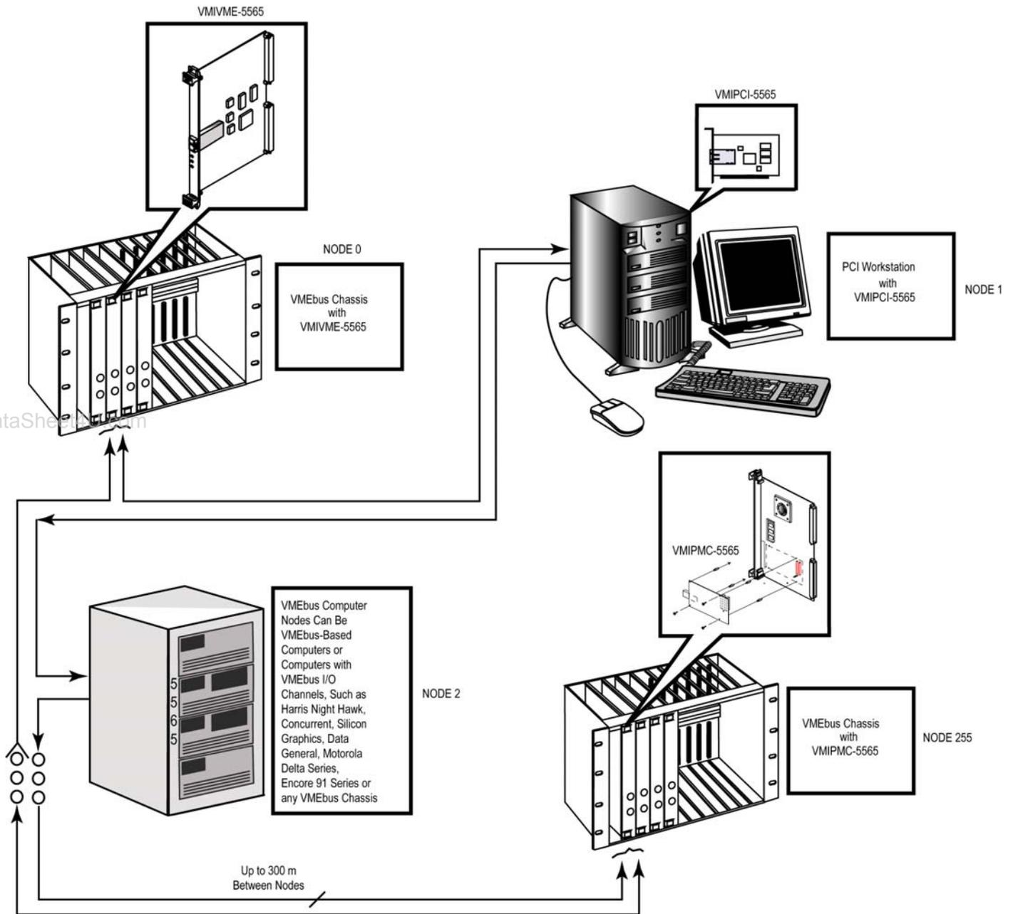
Figure 1. Network Example Using Reflective Memory System
