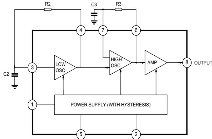
Note: R2, R3, C2 and C3 are parts externally mounted
