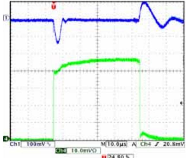
**SUPPLY VOLTAGE, FAST TURN ON ( $T_{RISE} = 10\mu\text{s}$ )**
