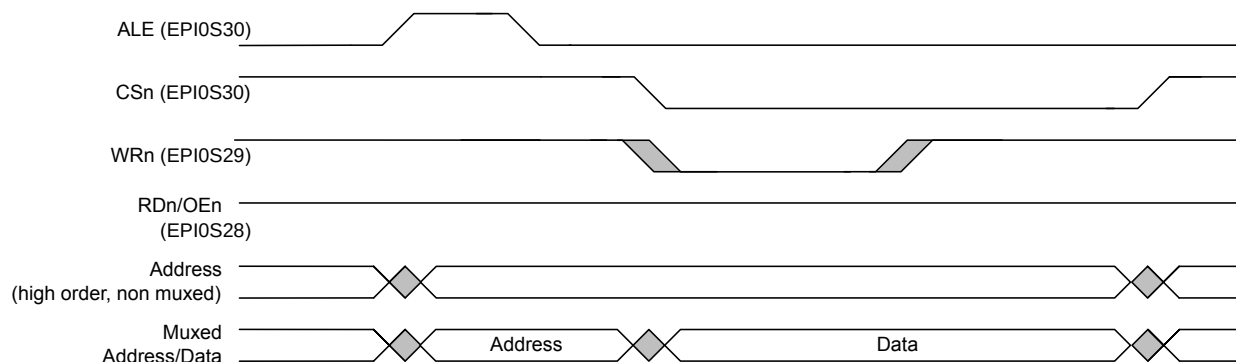
Figure 10-7. Host-Bus Write Cycle with Multiplexed Address and Data, MODE = 0x0, WRHIGH = 1, RDHIGH = 1
