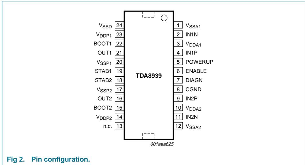
Fig 2. Pin configuration.
