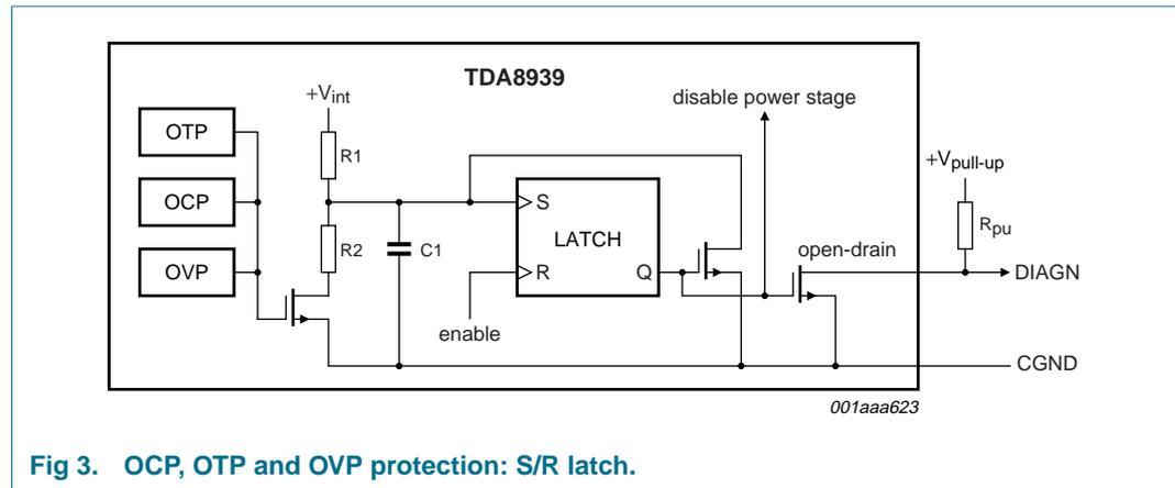
Fig 3. OCP, OTP and OVP protection: S/R latch.
