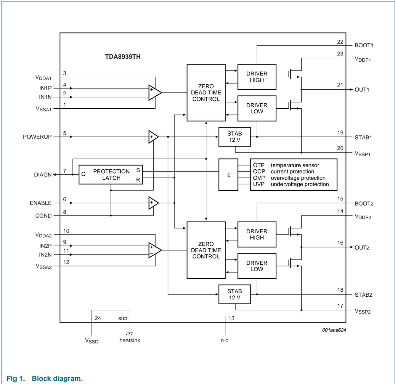
Fig 1. Block diagram.
