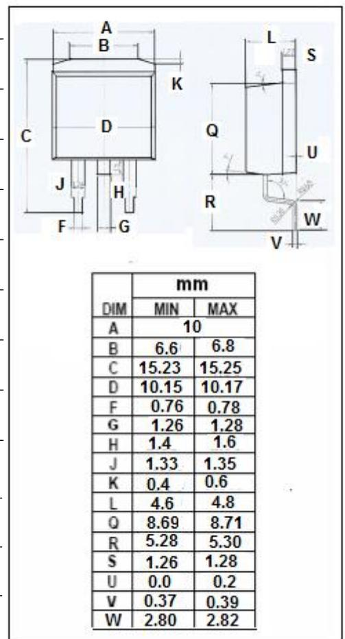
**isc N-Channel MOSFET Transistor**
