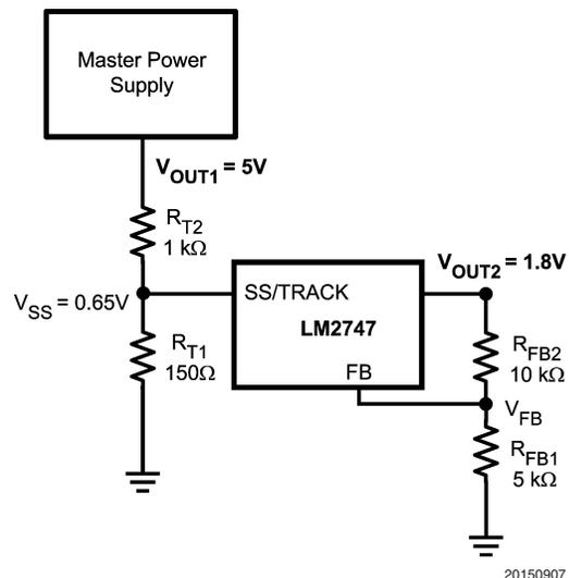
FIGURE 3. Tracking Circuit
