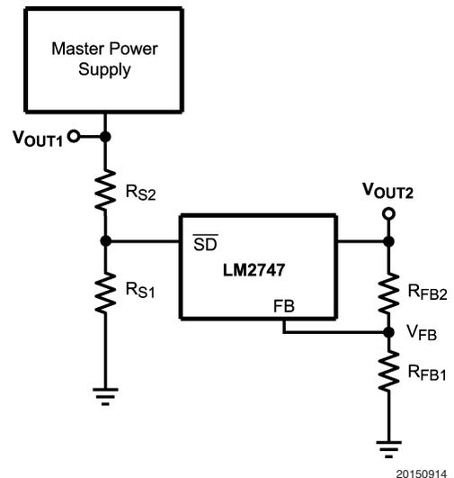
FIGURE 6. Sequencing Circuit
