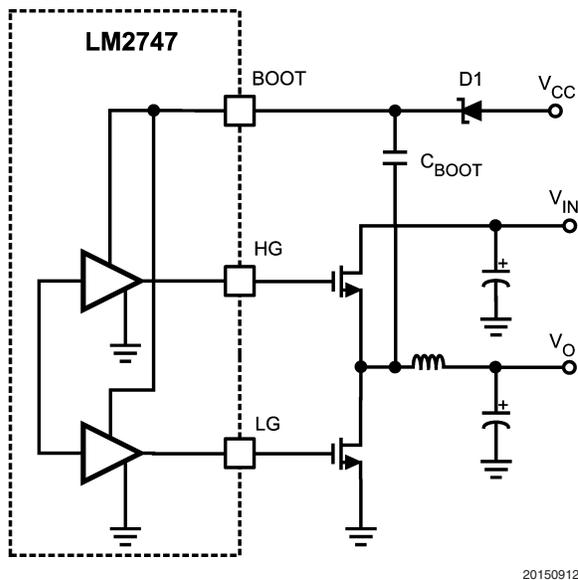
FIGURE 9. Basic Charge Pump (Bootstrap)
