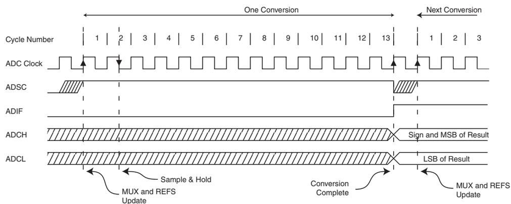
**Figure 22-6.** ADC Timing Diagram, Auto Triggerred Conversion
