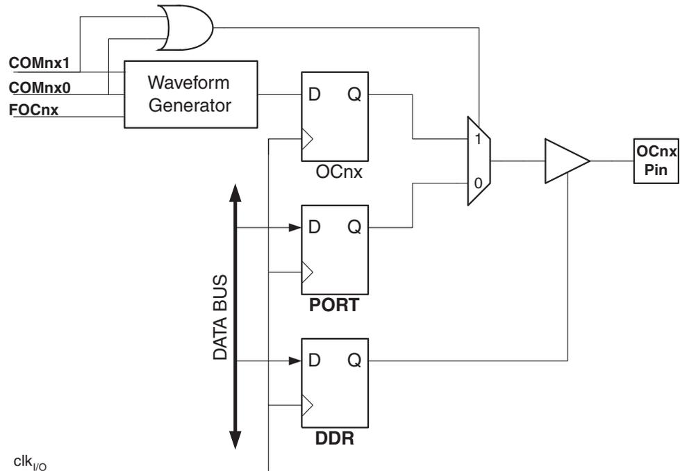
The general I/O port function is overridden by the Output Compare (OC2A) from the Waveform Generator if either of the COM2A1:0 bits are set. However, the OC2A pin direction (input or output) is still controlled by the Data Direction Register (DDR) for the port pin. The Data Direction Register bit for the OC2A pin (DDR\_OC2A) must be set as output before the OC2A value is visible on the pin. The port override function is independent of the Waveform Generation mode.
