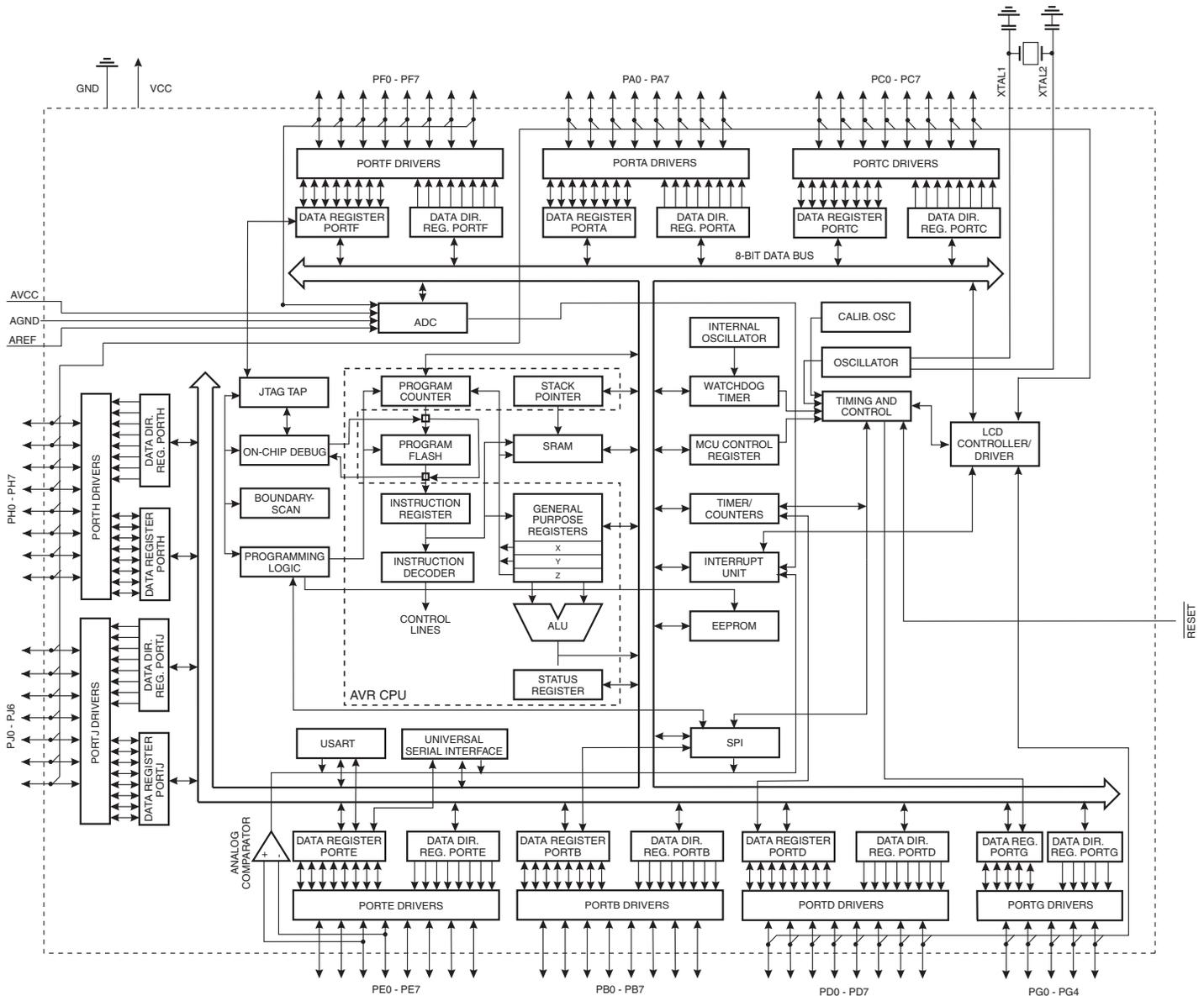
The Atmel® AVR® core combines a rich instruction set with 32 general purpose working registers. All the 32 registers are directly connected to the Arithmetic Logic Unit (ALU), allowing two independent registers to be accessed in one single instruction executed in one clock cycle. The resulting architecture is more code efficient while achieving throughputs up to ten times faster than conventional CISC microcontrollers.
