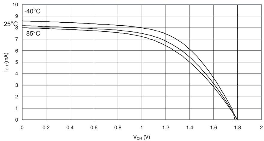
**Figure 29-27.** I/O Pin Sink Current vs. Output Voltage, Ports A, C, D, E, F, G, H, J
