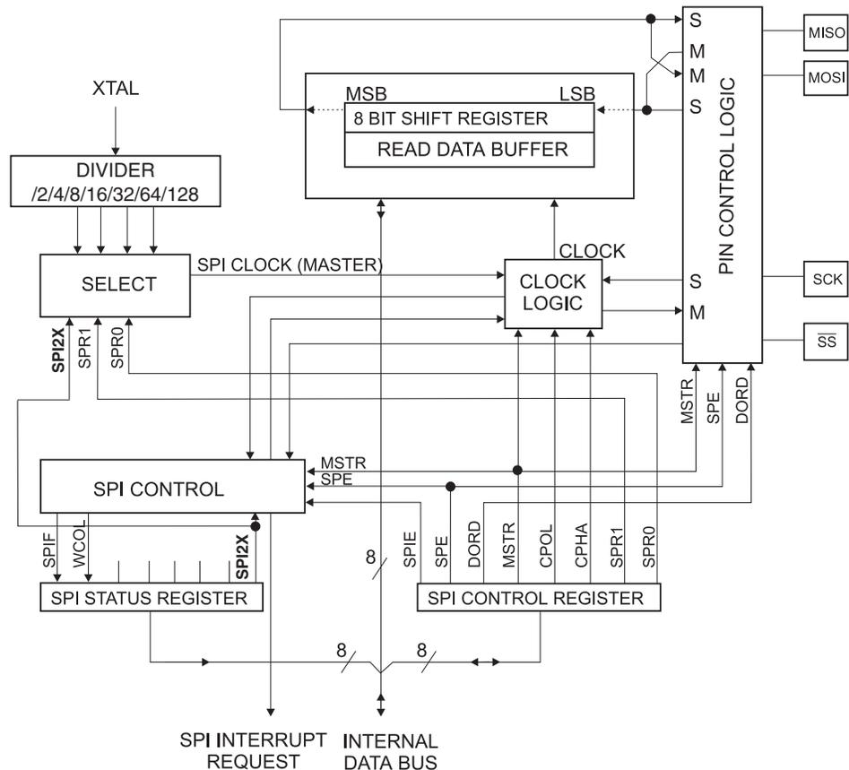
Note: 1. Refer to Figure 1-1 on page 2, and Table 13-6 on page 68 for SPI pin placement.
