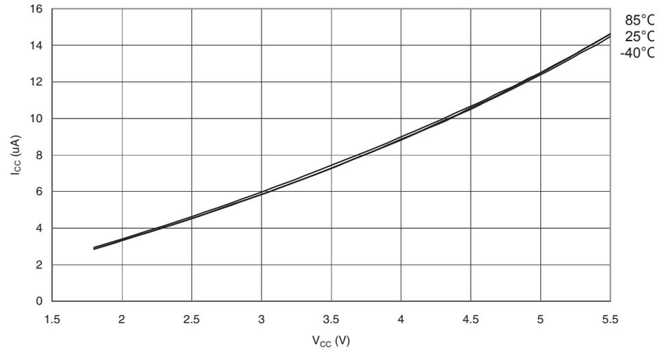
**Figure 29-54. Analog Comparator Current vs.  $V_{CC}$**
