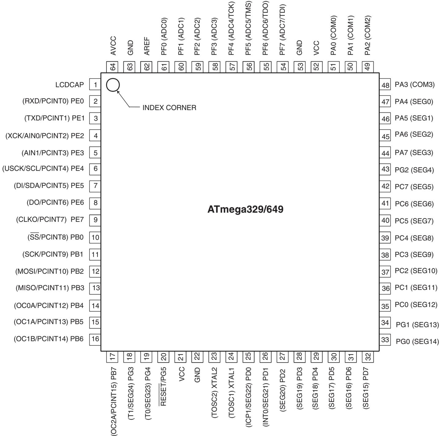
Note: The large center pad underneath the QFN/MLF packages is made of metal and internally connected to GND. It should be soldered or glued to the board to ensure good mechanical stability. If the center pad is left unconnected, the package might loosen from the board.
