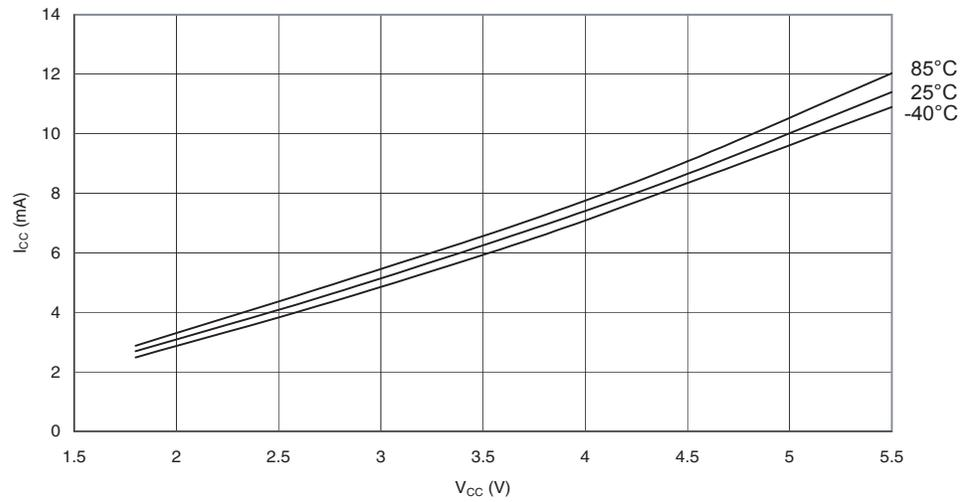
**Figure 29-4.** Active Supply Current vs.  $V_{CC}$
