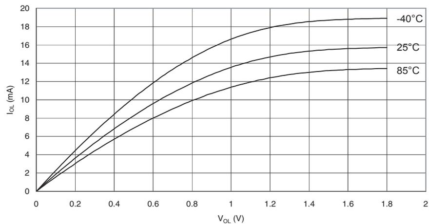
**Figure 29-29.** I/O Pin Sink Current vs. Output Voltage, Ports A, C, D, E, F, G, H, J
