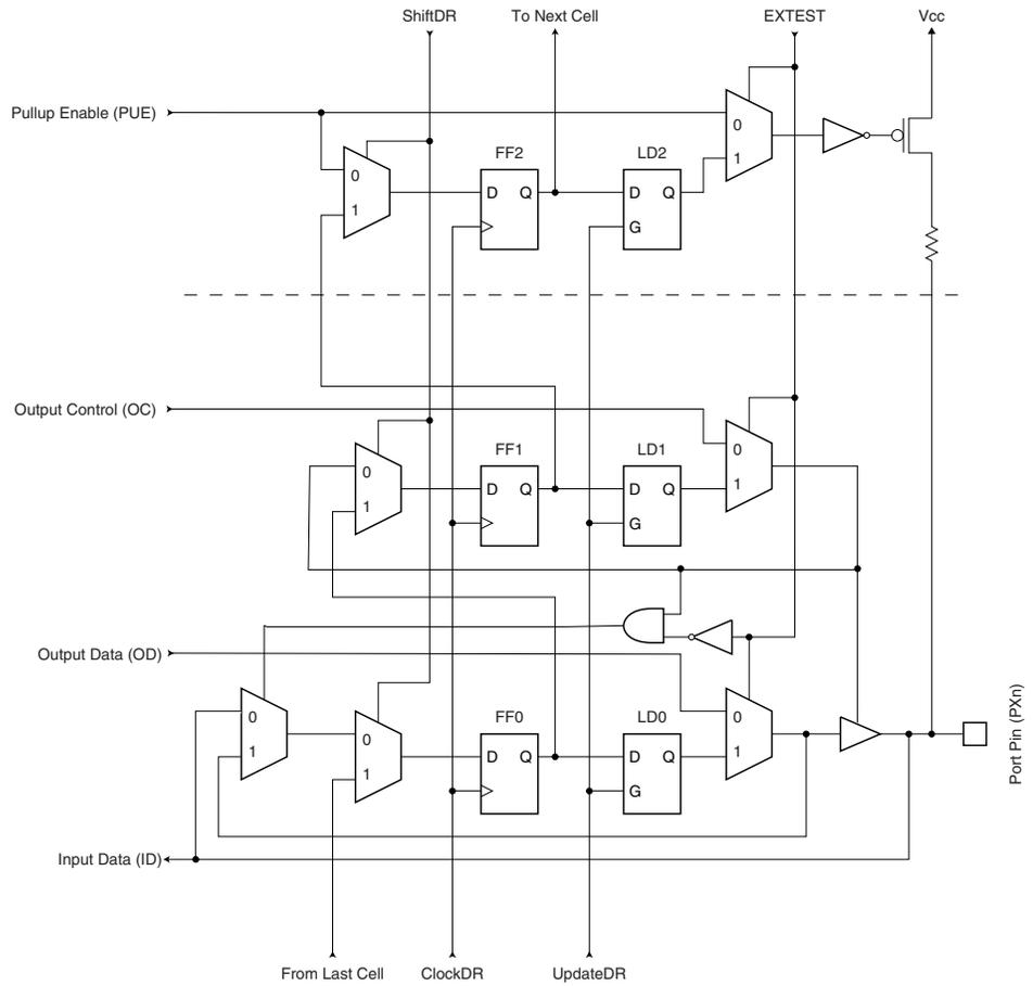
**Figure 25-4. General Port Pin Schematic Diagram**
