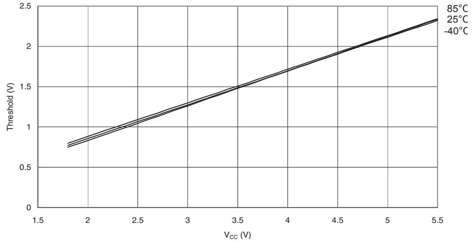
**Figure 29-38.** Reset Input Pin Hysteresis vs.  $V_{CC}$
