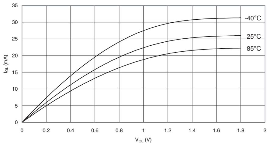
**Figure 29-32.** I/O Pin Sink Current vs. Output Voltage, Port B ( $V_{CC} = 1.8V$ )
