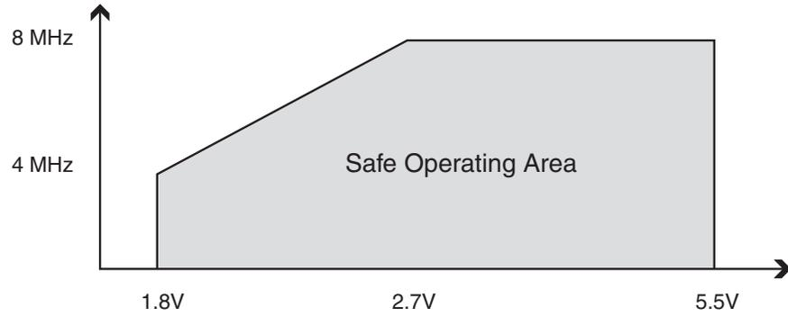
**Figure 28-2.** Maximum Frequency vs.  $V_{CC}$  (8 - 16MHz).
