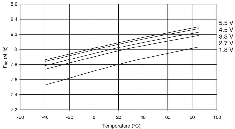
**Figure 29-47.** Calibrated 8MHz RC Oscillator Frequency vs.  $V_{CC}$
