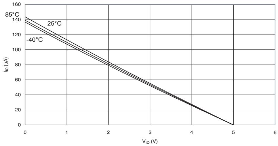
**Figure 29-16.** I/O Pin Pull-up Resistor Current vs. Input Voltage ( $V_{CC} = 2.7V$ )
