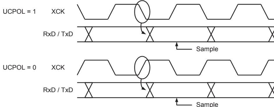
The UC POL<sub>n</sub> bit UCRSC selects which XCK clock edge is used for data sampling and which is used for data change. As [Figure 19-3](#) shows, when UC POL<sub>n</sub> is zero the data will be changed at rising XCK edge and sampled at falling XCK edge. If UC POL<sub>n</sub> is set, the data will be changed at falling XCK edge and sampled at rising XCK edge.
