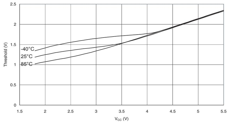
**Figure 29-37.** Reset Input Threshold Voltage vs.  $V_{CC}$  ( $V_{IL}$ , Reset Pin Read as “0”)
