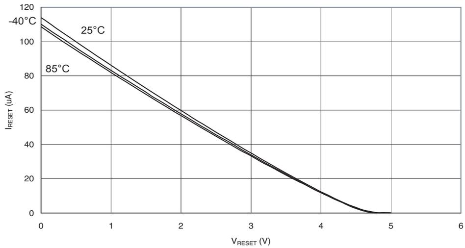
**Figure 29-19.** Reset Pull-up Resistor Current vs. Reset Pin Voltage ( $V_{CC} = 2.7V$ )
