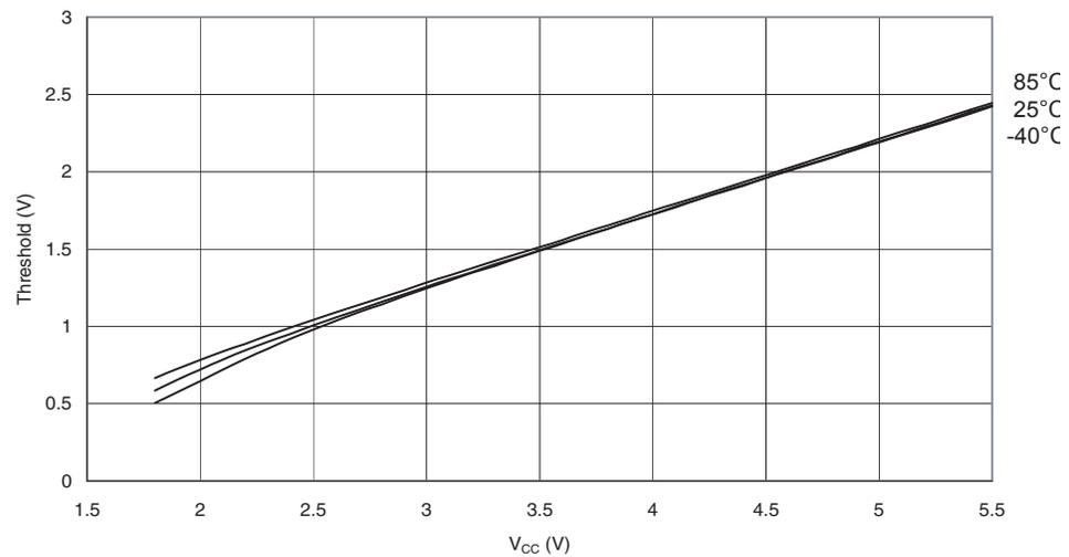
**Figure 29-35.** I/O Pin Input Hysteresis vs.  $V_{CC}$
