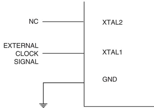
When this clock source is selected, start-up times are determined by the SUT Fuses as shown in [Table 8-10](#).
