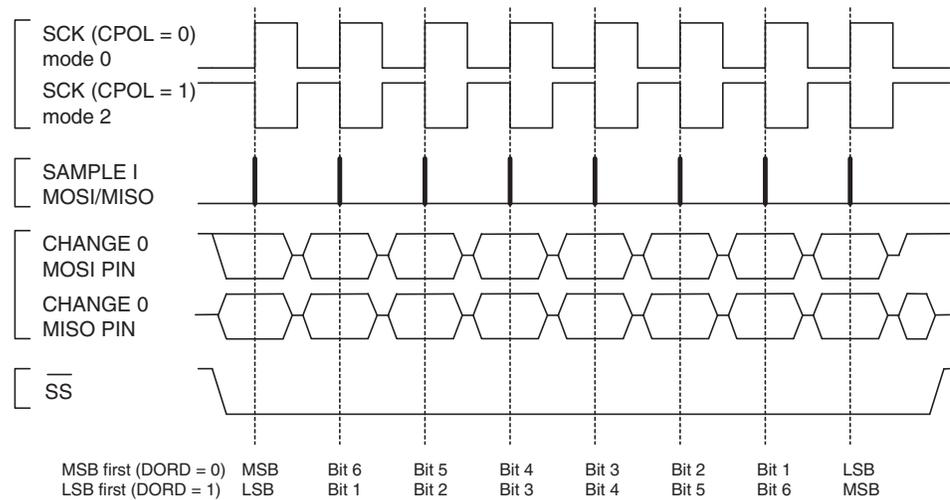
**Figure 18-4. SPI Transfer Format with CPHA = 1**
