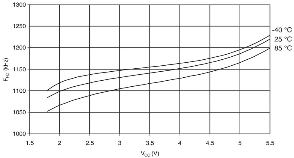
**Figure 29-46.** Calibrated 8MHz RC Oscillator Frequency vs. Temperature
