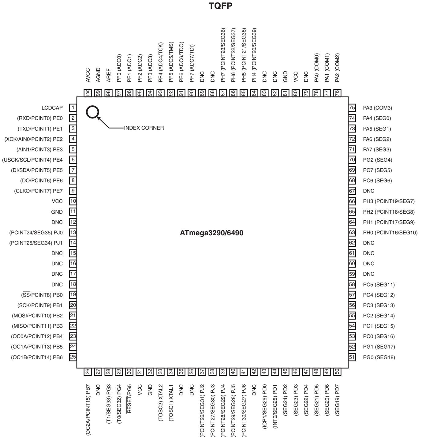
Figure 1-2. Pinout ATmega329/649
