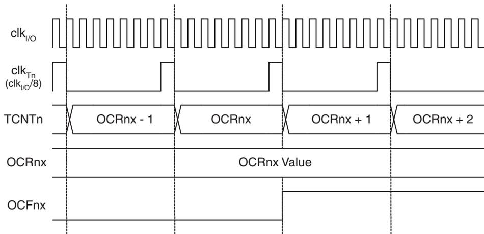
Figure 17-11 shows the setting of OCF2A and the clearing of TCNT2 in CTC mode.
