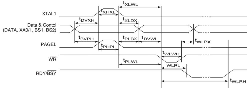
**Figure 27-8.** Parallel Programming Timing, Loading Sequence with Timing Requirements<sup>(1)</sup>
