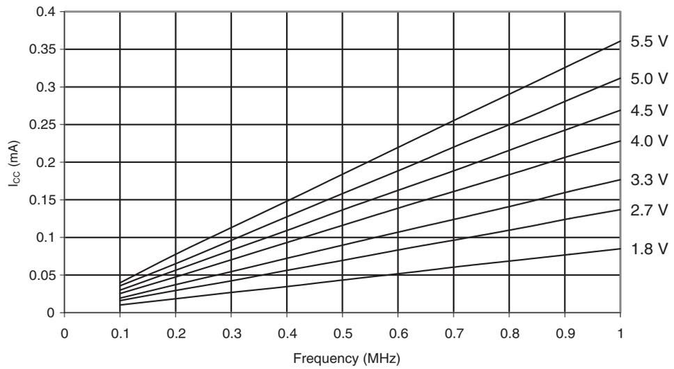
**Figure 29-7.** Idle Supply Current vs. Frequency (1 - 16MHz)
