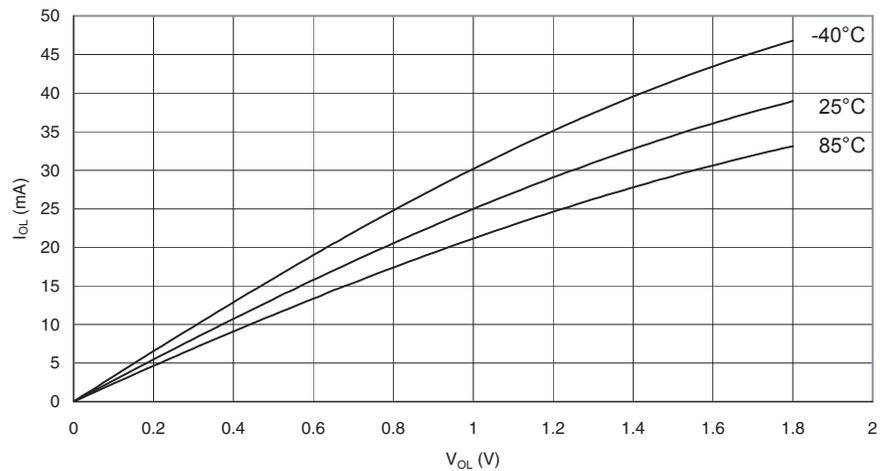
**Figure 29-28.** I/O Pin Sink Current vs. Output Voltage, Ports A, C, D, E, F, G, H, J
