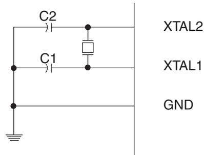
The Oscillator can operate in three different modes, each optimized for a specific frequency range. The operating mode is selected by the fuses CKSEL3..1 as shown in [Table 8-3](#).
