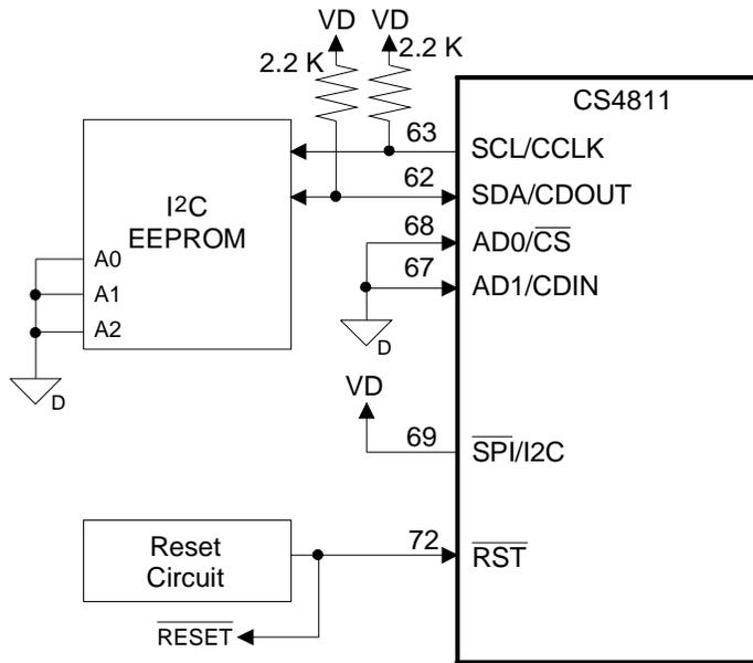
**Figure 4. Typical Connection Diagram, I<sup>2</sup>C Mode**
