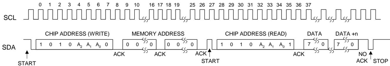
**Figure 10. Control Port Timing, I<sup>2</sup>C Master Mode Self-Boot**
