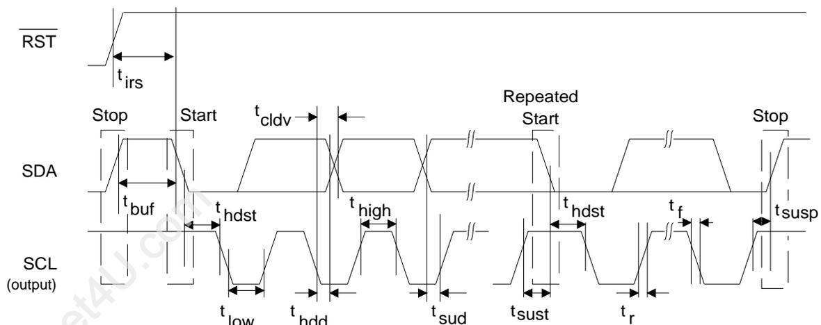
Figure 2. I<sup>2</sup>C Control Port Timing
