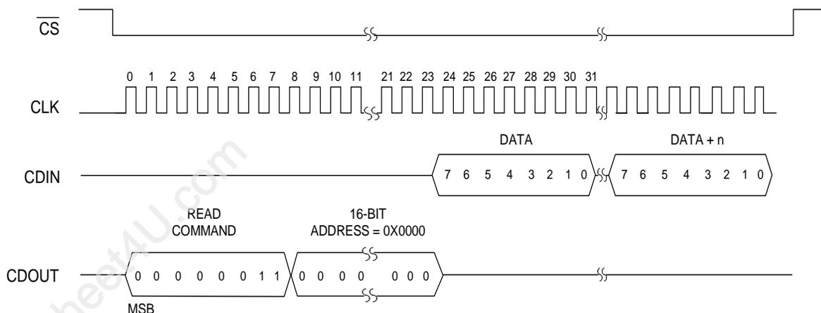
**Figure 9. Control Port Timing, SPI Master Mode Self-Boot**
