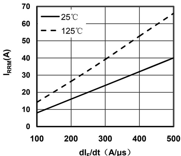
Figure 3. Reverse Recovery Current vs di<sub>F</sub>/dt
