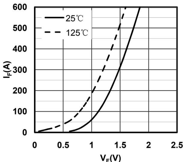
Figure 1. Forward Voltage Drop vs Forward Current
