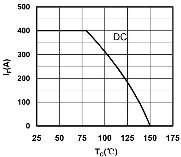
Figure 5. Forward current vs Case temperature
