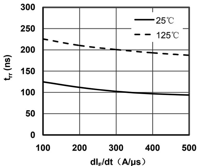
Figure 2. Reverse Recovery Time vs di<sub>F</sub>/dt
