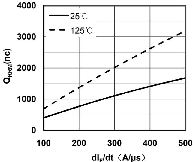
Figure 4. Reverse Recovery Charge vs di<sub>F</sub>/dt
