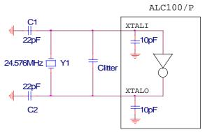
Fig-2 Clitter due to PCB Trace
