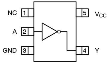
Figure 2. SC-88A and SC-74A (Top View)
