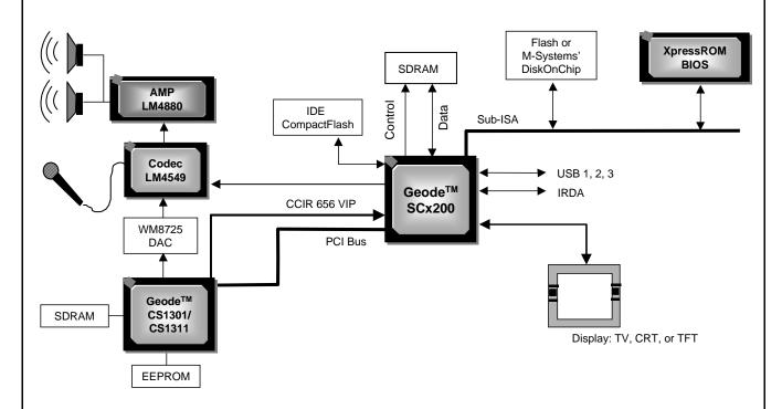
Figure 1-1. System Block Diagram
