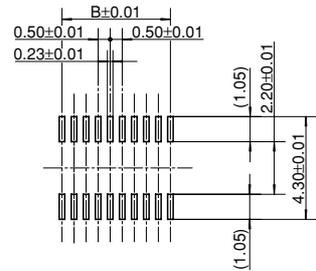
\* See the dimension table for more information on the B dimension of the socket and header.
