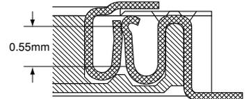
**5. The lower connector bottom surface construction prevents contact and shorts between the PCB and metal terminals.**
