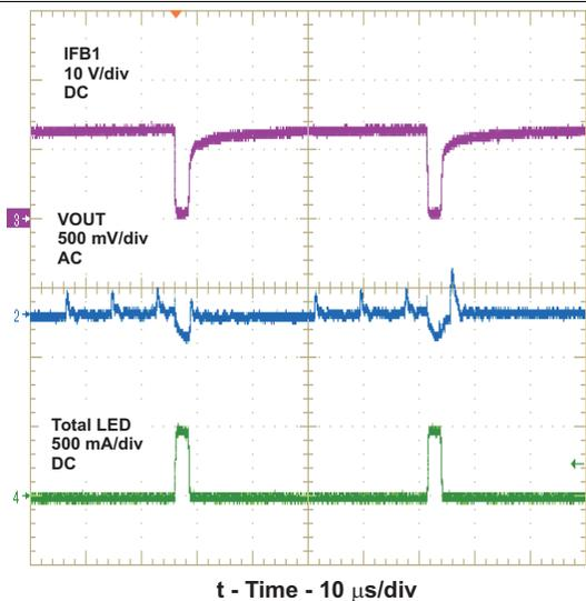
Figure 5. Dimming Waveforms
