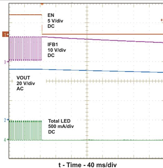
Figure 7. Shutdown Waveform
