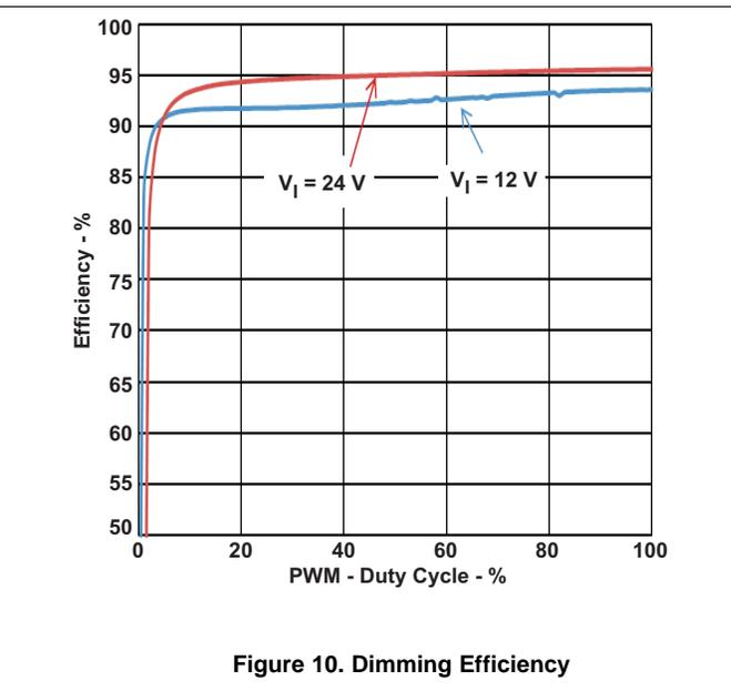
Figure 10. Dimming Efficiency
