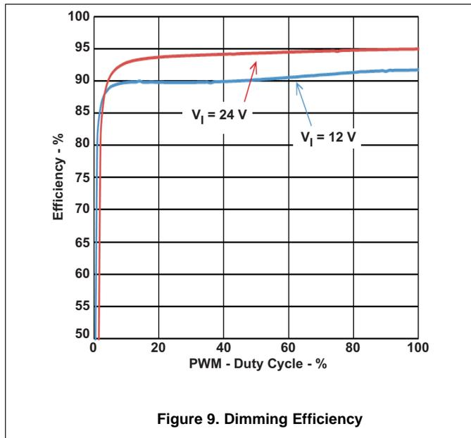
Figure 9. Dimming Efficiency
