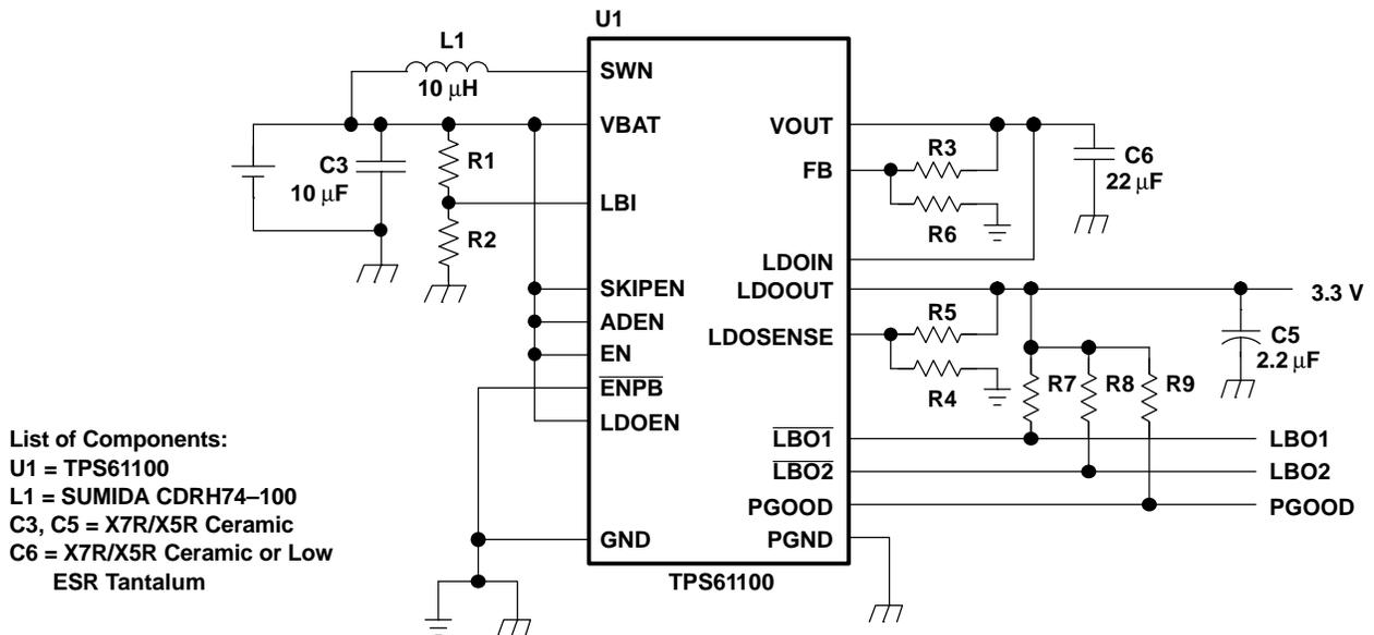
Figure 33. Single Output Using LDO as Filter
