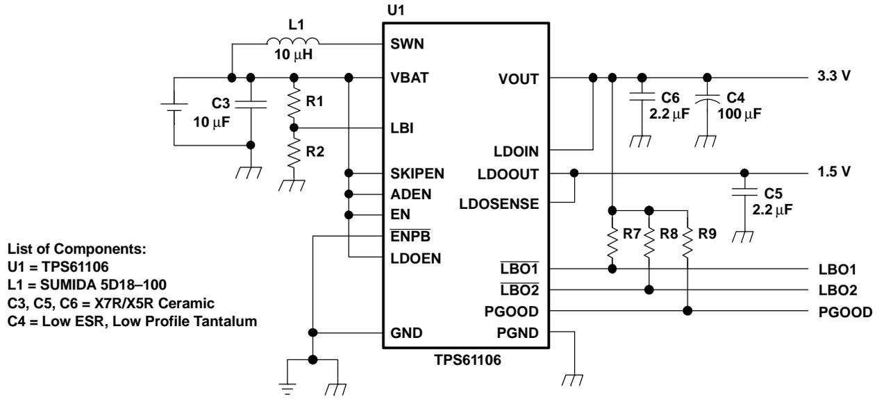
Figure 30. Low Profile Solution, Maximum Height 1,8 mm
