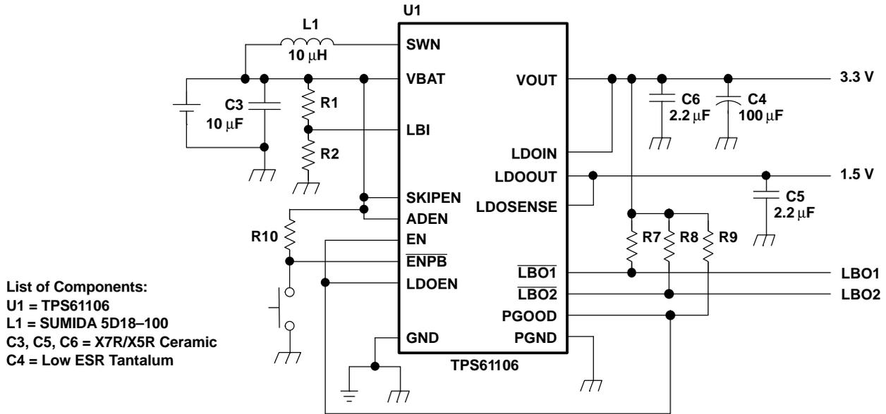
Figure 34. Simple Solution Using a Pushbutton for Start-Up
