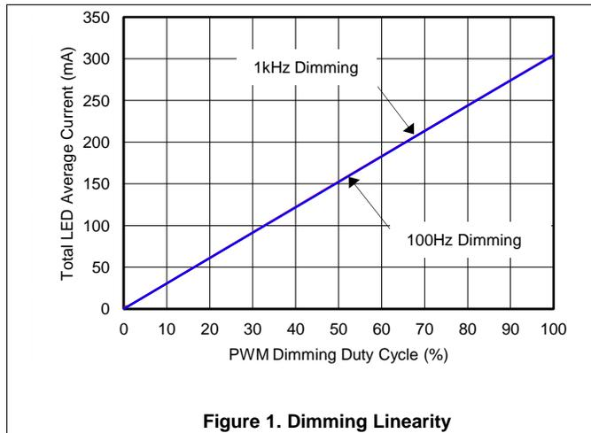
**Figure 1. Dimming Linearity**
