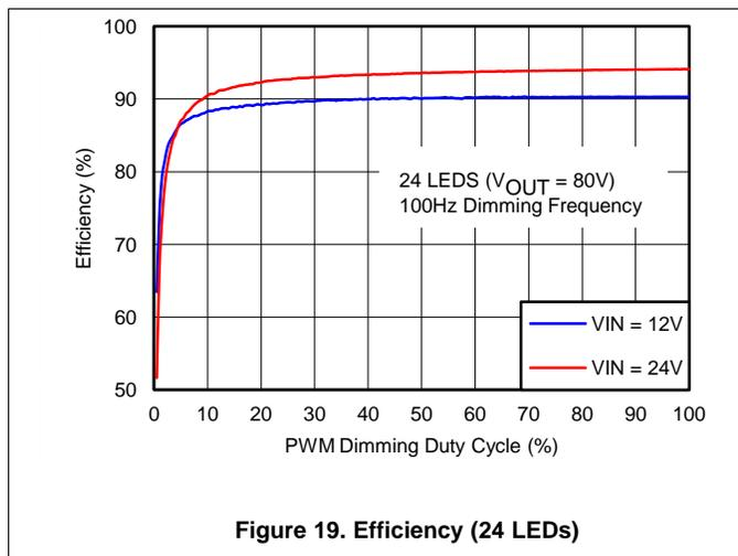
Figure 19. Efficiency (24 LEDs)
