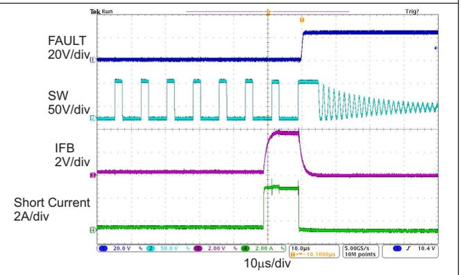
Figure 14. LED String Short Protection (100% Dimming)
