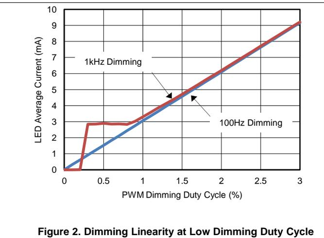
**Figure 2. Dimming Linearity at Low Dimming Duty Cycle**
