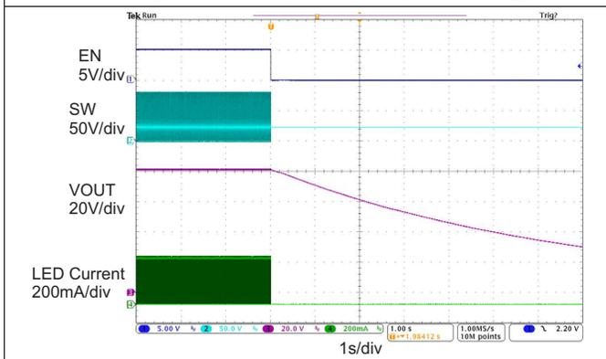
Figure 9. Shutdown Waveform (1% Dimming)
