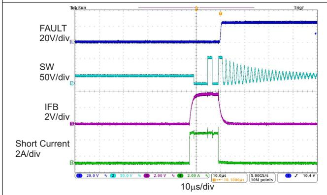
Figure 13. LED String Short Protection (1% Dimming)
