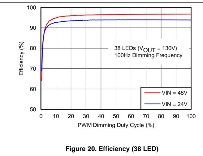
Figure 20. Efficiency (38 LED)
