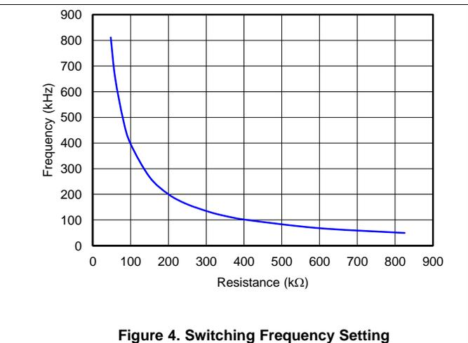
**Figure 4. Switching Frequency Setting**
