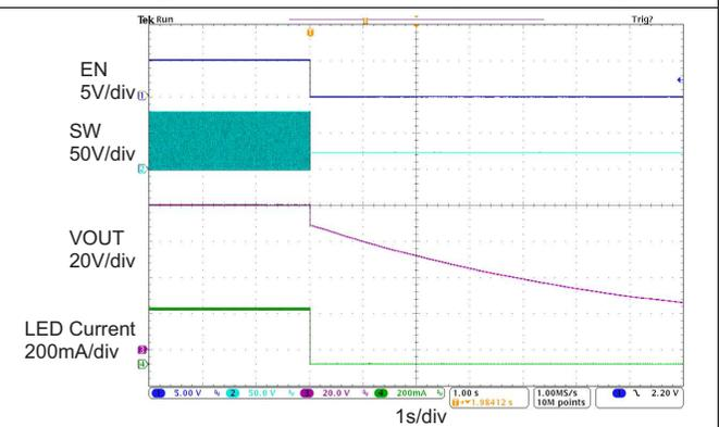
Figure 10. Shutdown Waveform (100% Dimming)
