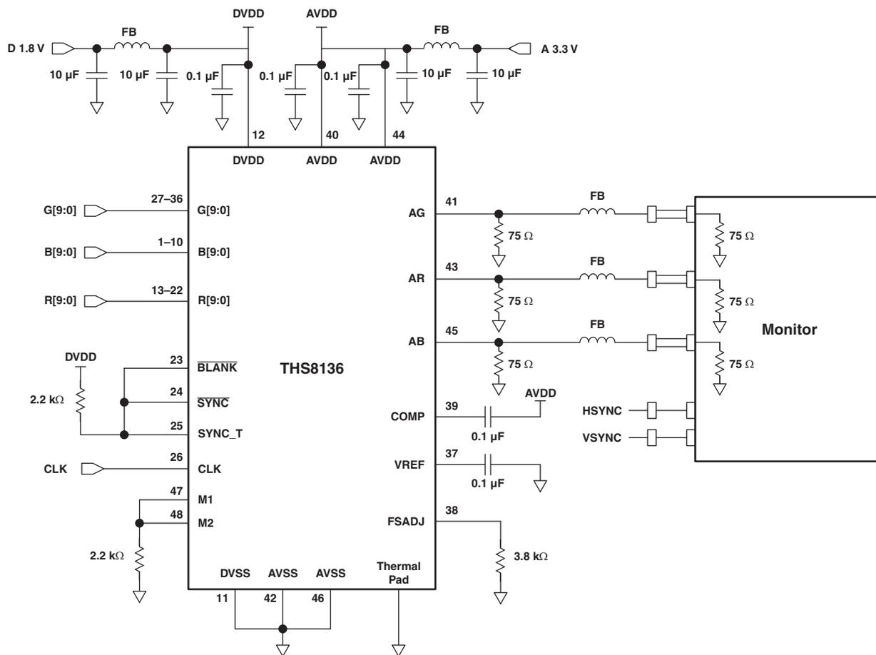
NOTE: System level ESD protection is not included in this application circuit, but it is highly recommended on the analog RGB outputs.
