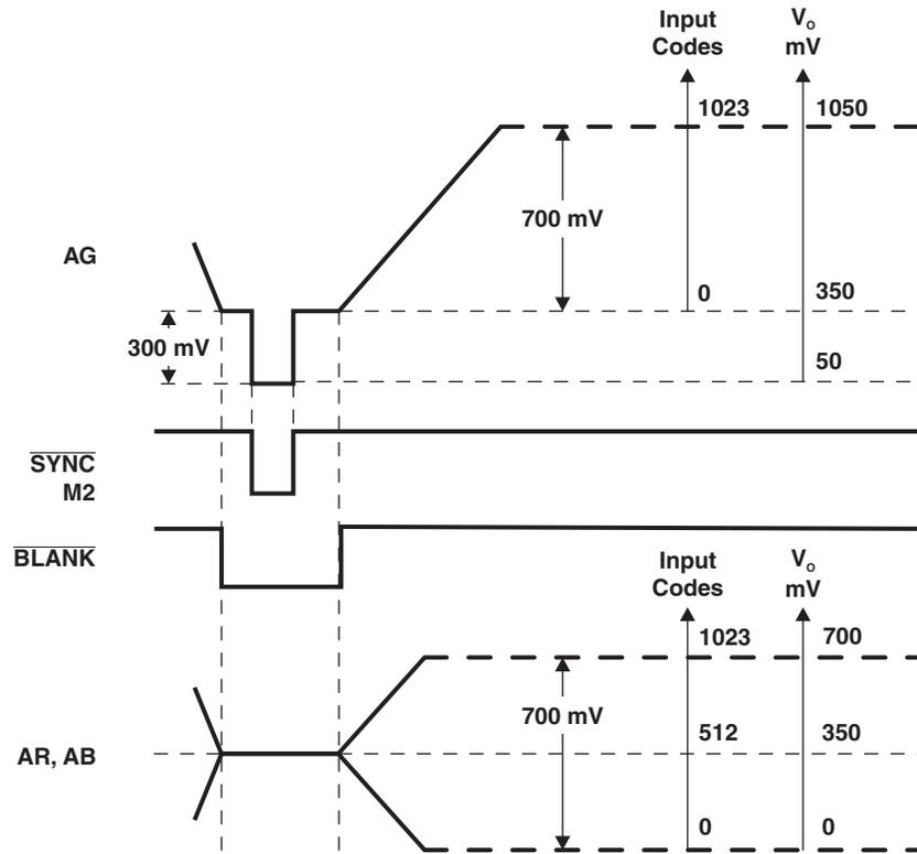
NOTE:  $R_{FS}$  chosen for 700-mV output.
