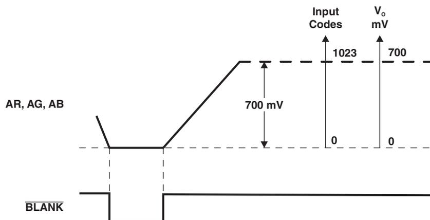
NOTE:  $\overline{\text{BLANK}}$  = High in applications not requiring a forced blank level.
