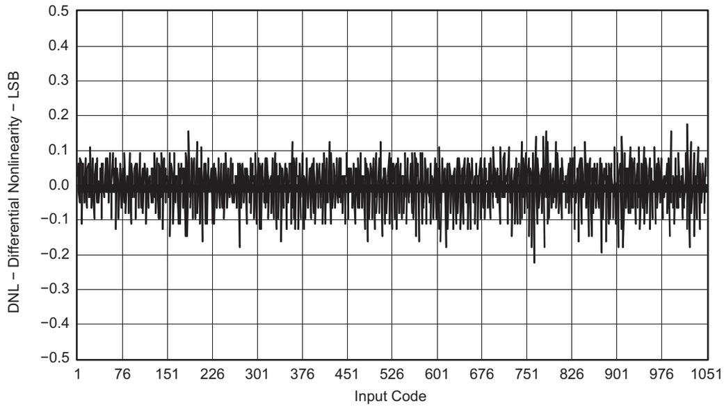
**Figure 13. DNL, Generic DAC Mode (1.3-V Output Compliance)**
