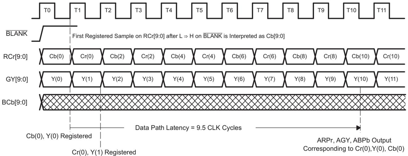
**Figure 8. Input Format and Latency YCbCr 4:2:2 2x10-Bit Mode**
