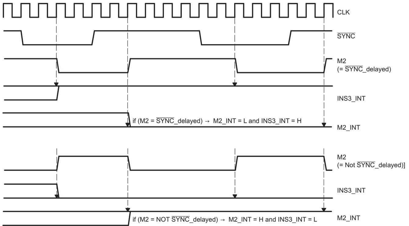
**Figure 6. Generating INS3\_INT and M2\_INT From M2**
