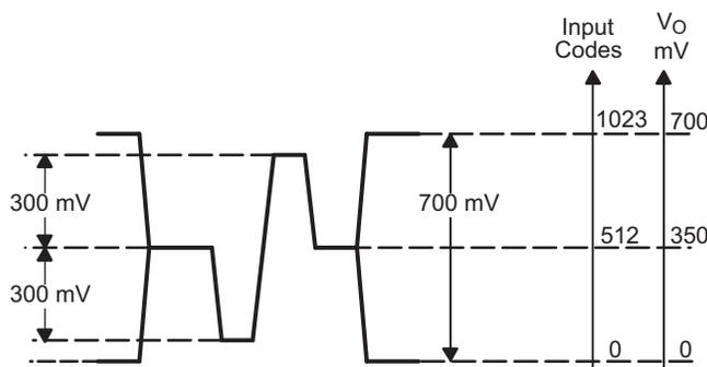
Figure 2. CbCr Outputs, Full-Scale Input Code Range
