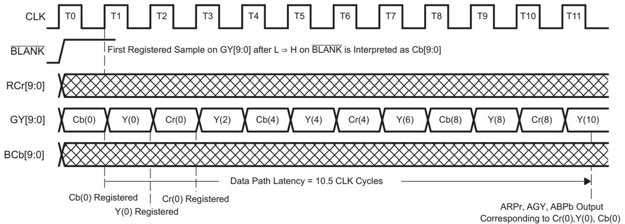
**Figure 9. Input Format and Latency YCbCr 4:2:2 1x10-Bit Mode**
