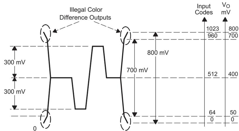
Figure 4. CbCr Outputs, Reduced-Scale Input Code Range
