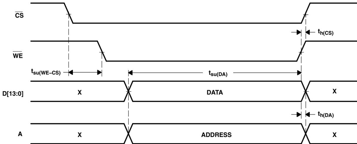
**Figure 3. Write Timing**
