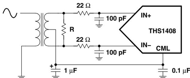
**Figure 17. Transformer Coupled**
