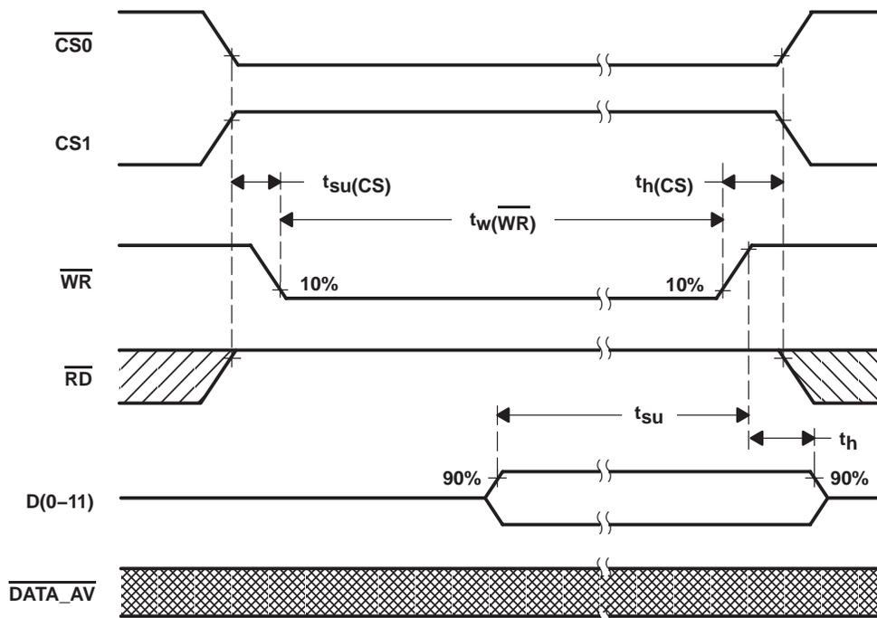
**Figure 16. Write Timing Diagram Using  $\overline{WR}$  ( $\overline{WR}$ -controlled)**
