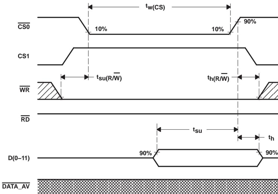
**Figure 14. Write Timing Diagram Using  $\overline{R/\overline{W}}$  ( $\overline{CS0}$ -controlled)**
