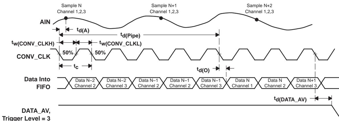
**Figure 4. Timing of Continuous Conversion Mode (3-channel operation)**
