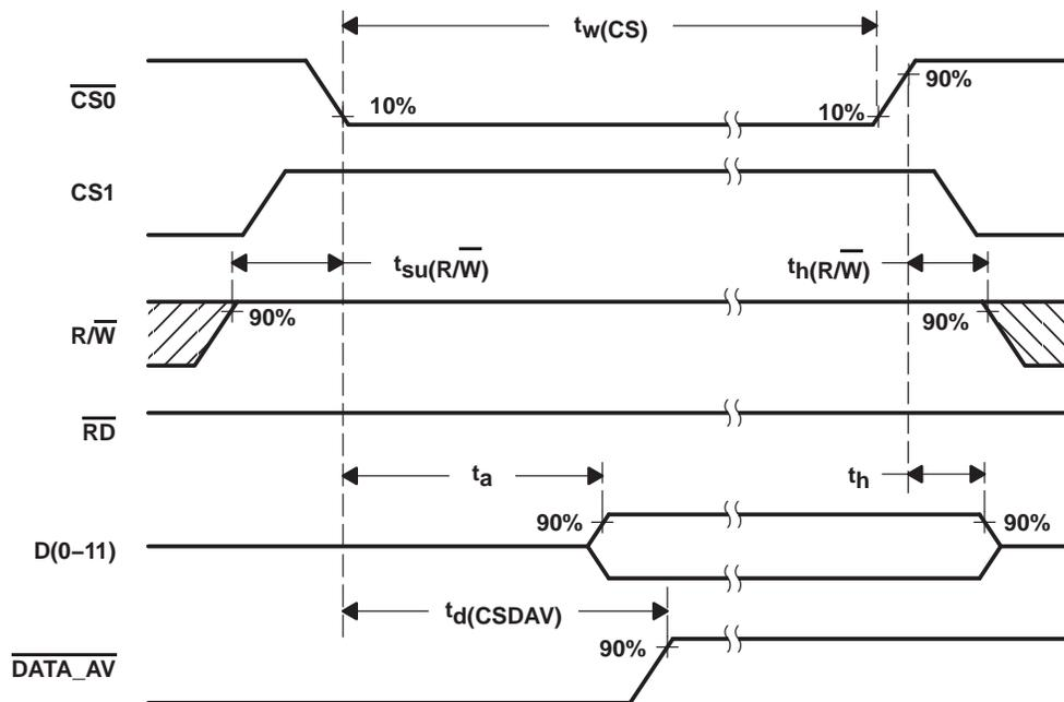
**Figure 13. Read Timing Diagram Using  $\overline{R/\overline{W}}$  ( $\overline{CS0}$ -controlled)**
