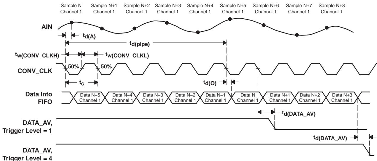
Figure 2. Timing of Continuous Conversion Mode (1-channel operation)
