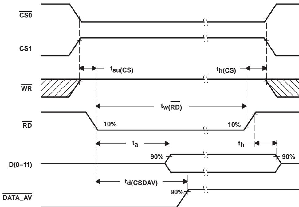
**Figure 15. Read Timing Diagram Using  $\overline{RD}$  ( $\overline{RD}$ -controlled)**
