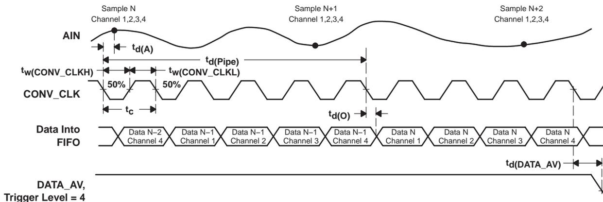
**Figure 5. Timing of Continuous Conversion Mode (4-channel operation)**
