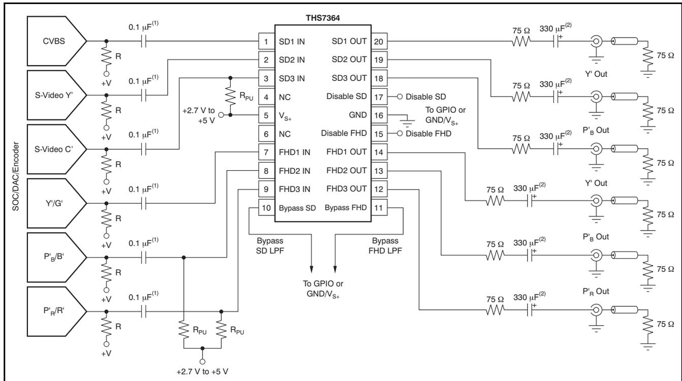
(1) AC-coupled input is shown in this example. DC-coupling is also allowed as long as the DAC output voltage is within the allowable linear input and output voltage range of the THS7364. To apply dc-coupling, remove the 0.1- $\mu$ F input capacitors and the  $R_{PU}$  pull-up resistors along with connecting the DAC termination resistors (R) to ground.
