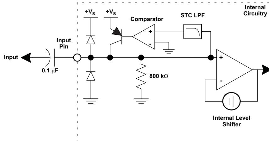
**Figure 6. Equivalent AC Sync-Tip Clamp Input Circuit**
