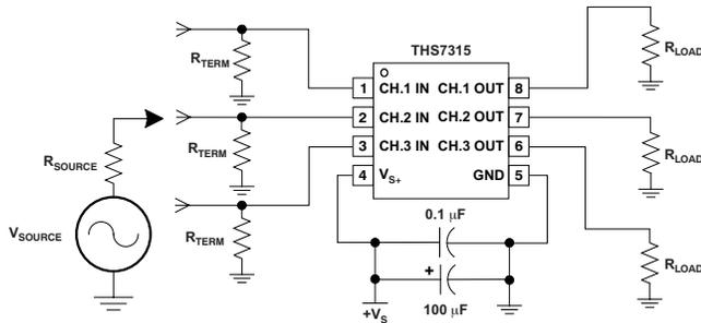
Figure 1. DC-Coupled Input and Output Test Circuit
