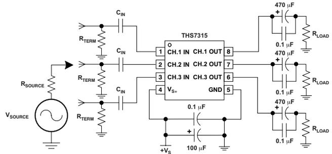
Figure 2. AC-Coupled Input and Output Test Circuit
