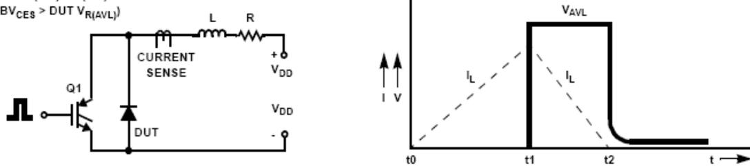
**Figure 2. Unclamped Inductive Switching Test Circuit & Waveform**
