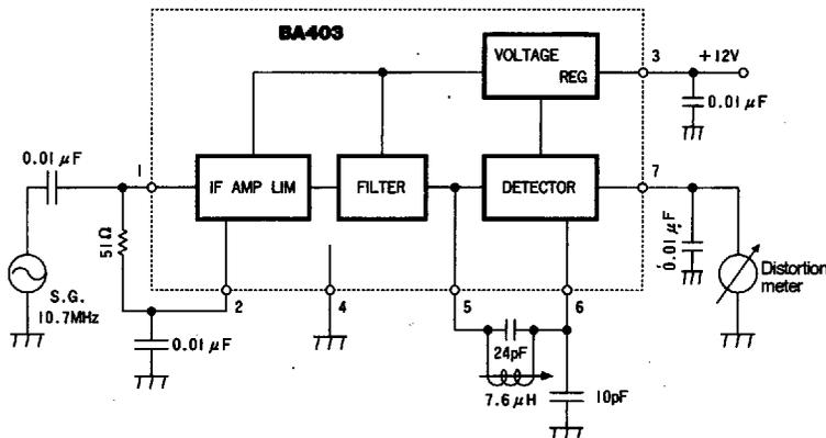
Figure 2 BA403 equivalent circuit
