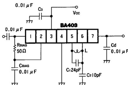
**C<sub>BIAS</sub>:** This is the bypass capacitor for the self-biasing, differential amplifier. It is used to ground the IF carriers. If C<sub>1</sub> is 24 pF and C<sub>2</sub> is 10 pF, the output level is a standard 500 mV<sub>rms</sub>.
