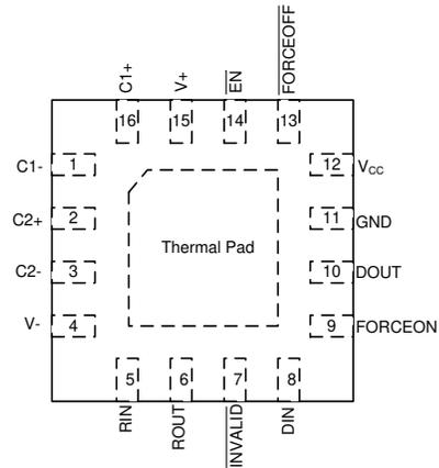
**Figure 5-2. 16-pin VQFN (RGT) Package, Top View**
