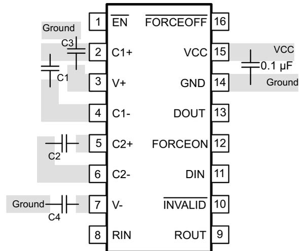
**Figure 10-1. Layout Diagram**
