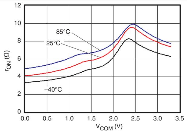
Figure 2.  $r_{on}$  vs  $V_{COM}$  ( $V_+ = 3.3$  V)
