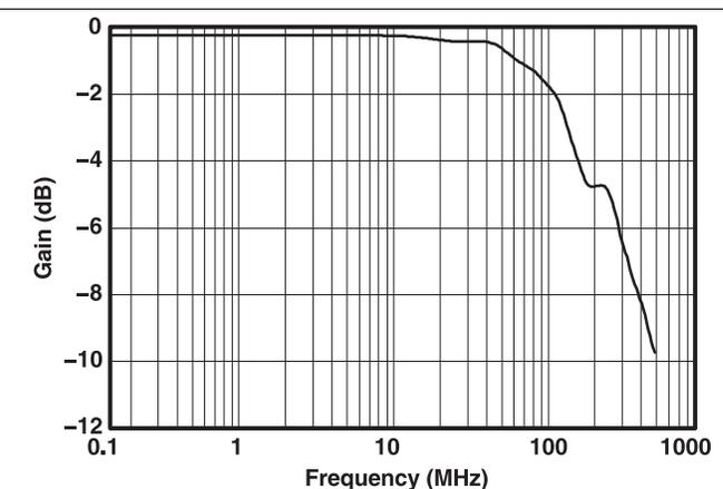
Figure 8. Bandwidth (Gain vs Frequency) ( $V_+ = 3.3$  V)
