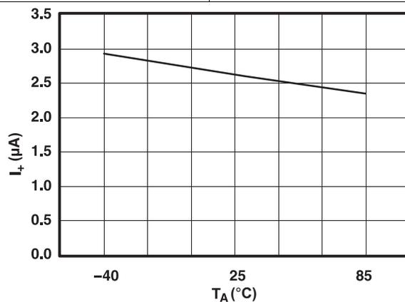
Figure 11. Power-Supply Current vs Temperature ( $V_+ = 3.6$  V)
