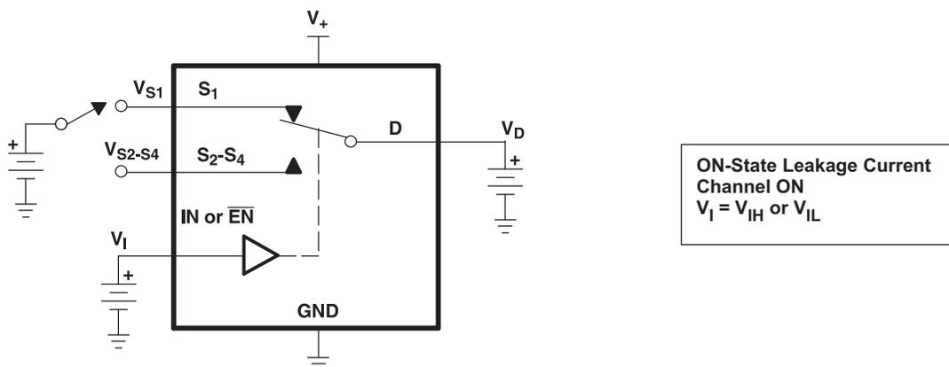
**Figure 14. ON-State Leakage Current ( $I_{D(ON)}$ ,  $I_{S(ON)}$ )**
