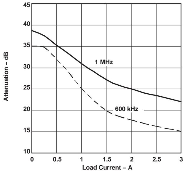
**Figure 34.  $\pi$ -Filter Attenuation vs. Load Current**
