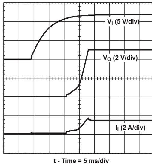
Figure 29. Power-Up Waveforms
