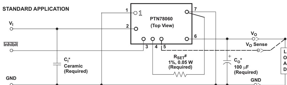
\*See the *Application Information* section for capacitor recommendations. The minimum input capacitance is 2.2 µF for PTN78060W, and 14.1 µF (3 x 4.7 µF) for PTN78060H.
