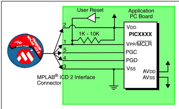
Although pin 2 (VDD) can supply a limited amount of power to the target application under certain conditions, for the purposes of these descriptions, pins 2 and 3 (VSS) are omitted. They are shown on the diagram for completeness, but in the following descriptions only three lines are active and relevant to core MPLAB ICD 2 operation:  $VPP/MCLR$ , PGC and PGD.
