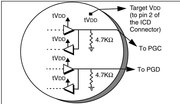
If MPLAB ICD 2 does not have voltage on its VDD line (pin 2 of the ICD connector) it will not operate. Using a scope, communications on PGC and PGD with a full target VDD to VSS peak-to-peak waveform should be seen. VPP should show +12, +5 and 0V levels depending upon the operation being performed. Signals should be seen on those lines only after performing an MPLAB ICD 2 function from the MPLAB user interface. Otherwise, all these lines should be idle and noise free.
