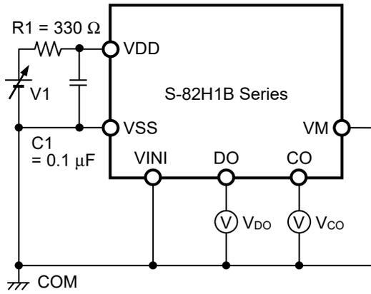
**Figure 3 Test Circuit 1**
