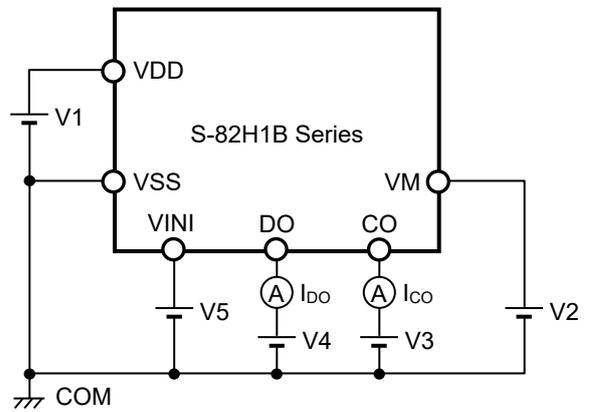
**Figure 6 Test Circuit 4**
