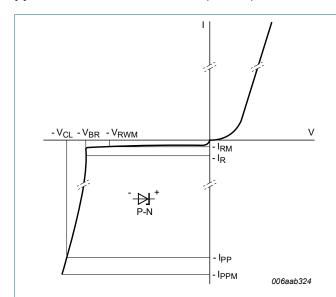
Fig. 3. V-I characteristics for a unidirectional TVS protection diode
