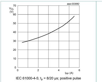
Fig. 5. Dynamic resistance with positive clamping; typical values
