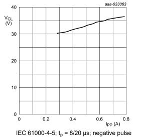
Fig. 6. Dynamic resistance with negative clamping; typical values
