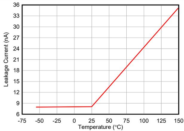
Figure 6-3. Temperature vs Leakage Current
