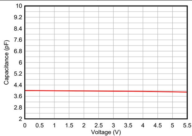
Figure 6-5. Bias Voltage vs Capacitance
