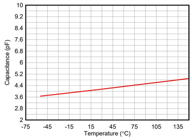
Figure 6-4. Temperature vs Capacitance
