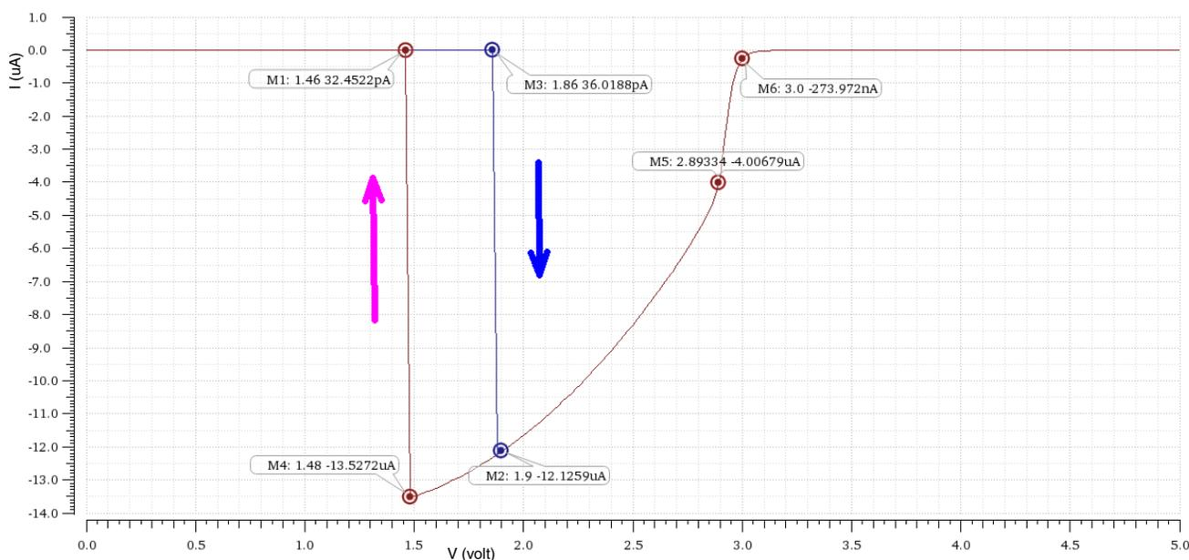
**Figure 5.  $I_{IN}/I_{OZ}$  vs.  $V_{IN}$  (typical; pull-up disabled) (design simulation)****8.3.4 Power mode operating behaviors**
