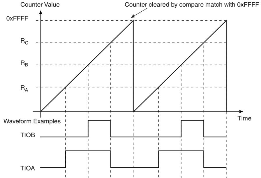
**Figure 91.** WAVSEL= 00 with trigger
