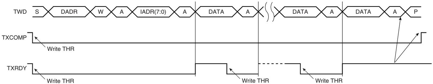
**Figure 32. Master Read with One, Two or Three Bytes Internal Address and One Data Byte**
