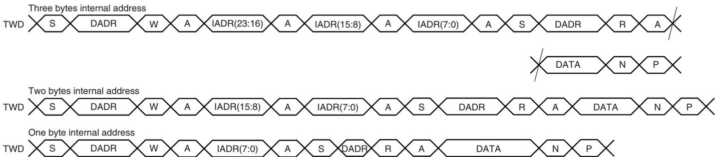
**Figure 33.** Master Read with One Byte Internal Address and Multiple Data Bytes
