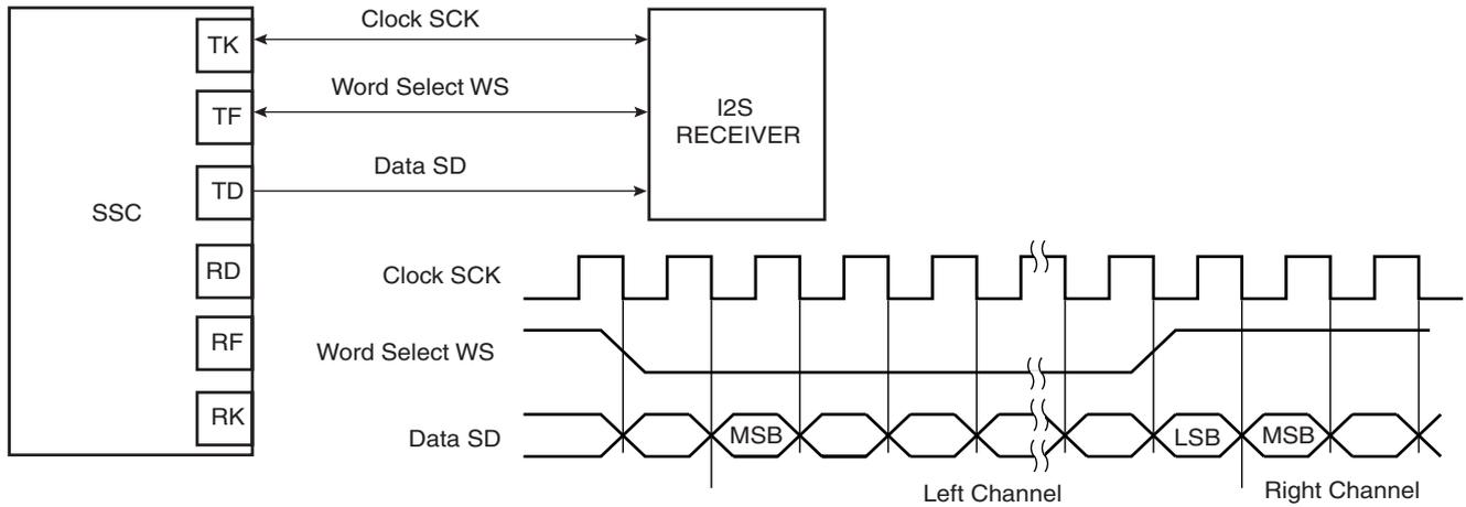
**Figure 83.** Codec Application Block Diagram
