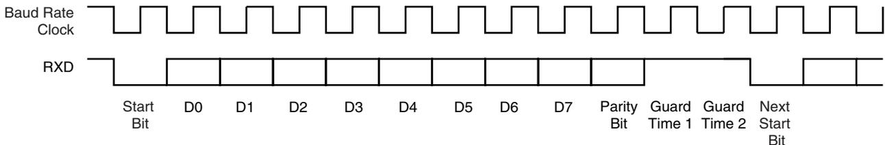
**Figure 57. T = 0 Protocol with Parity Error**
