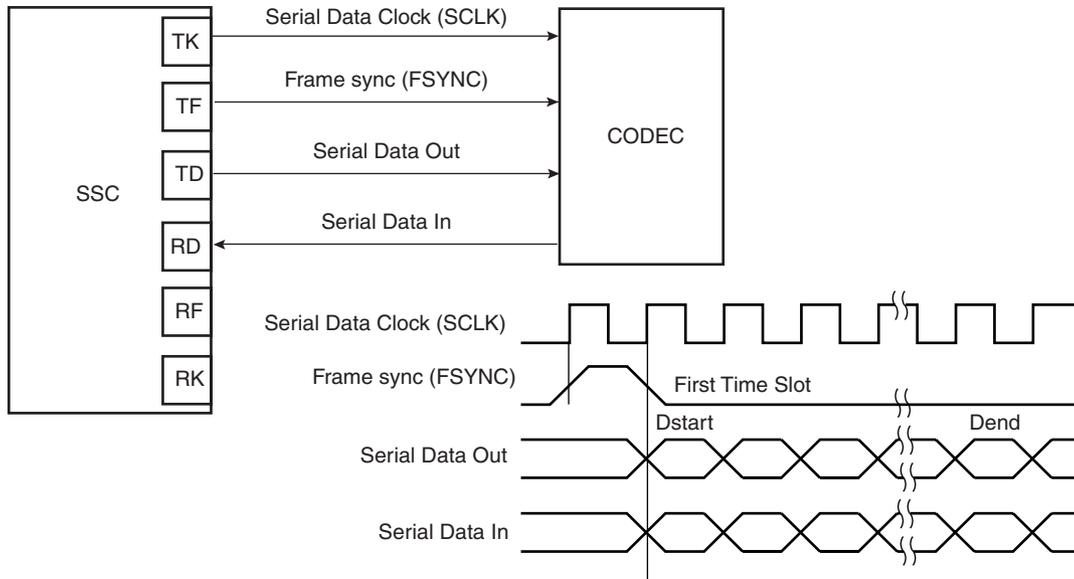
**Figure 84.** Time Slot Application Block Diagram
