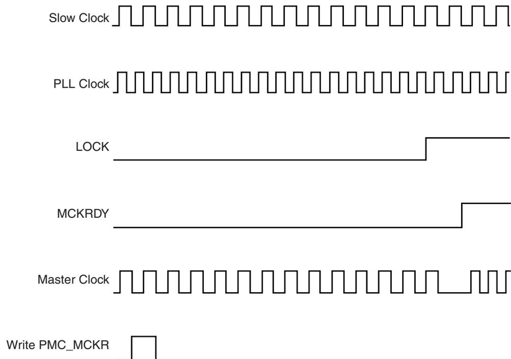
**Figure 56.** Switch Master Clock from Main Clock to Slow Clock
