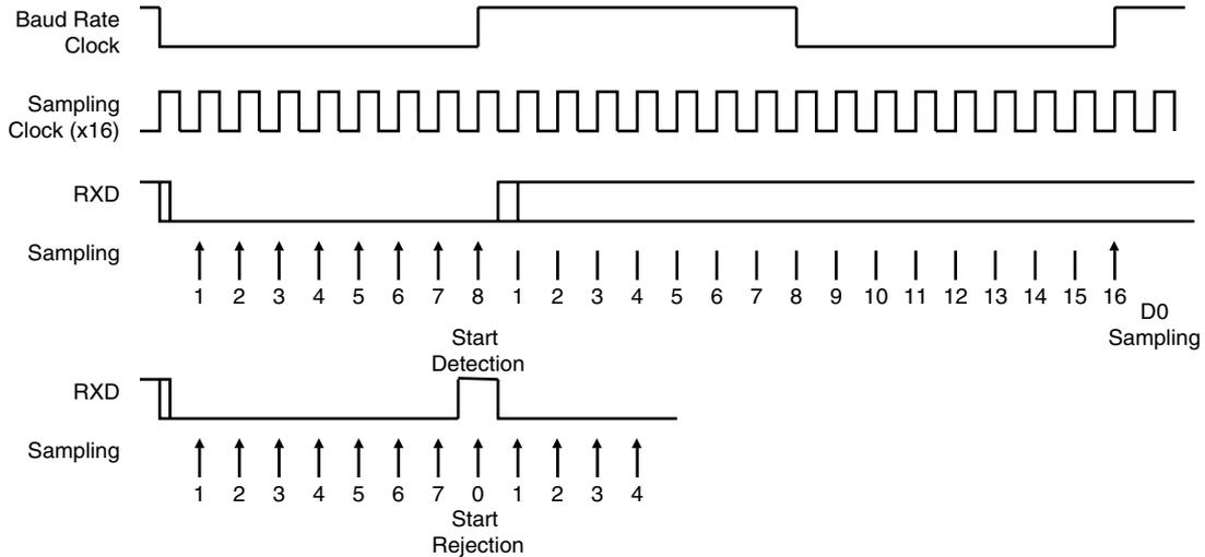
**Figure 44. Asynchronous Character Reception**
