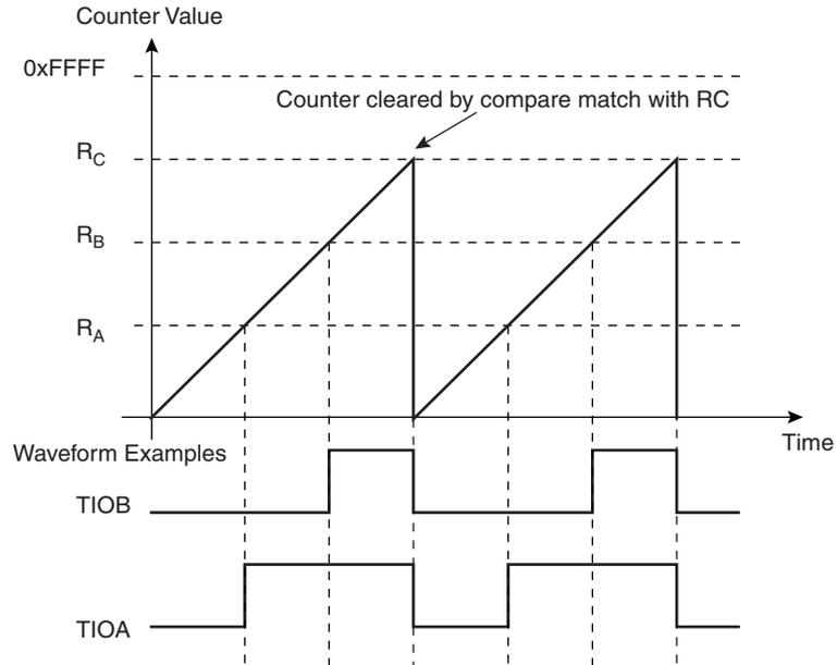
**Figure 93. WAVSEL = 10 With Trigger**
