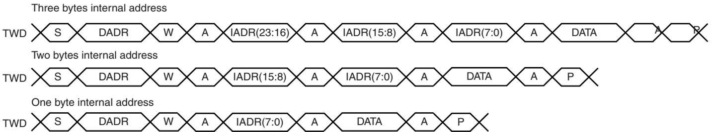
**Figure 31. Master Write with One Byte Internal Address and Multiple Data Bytes**
