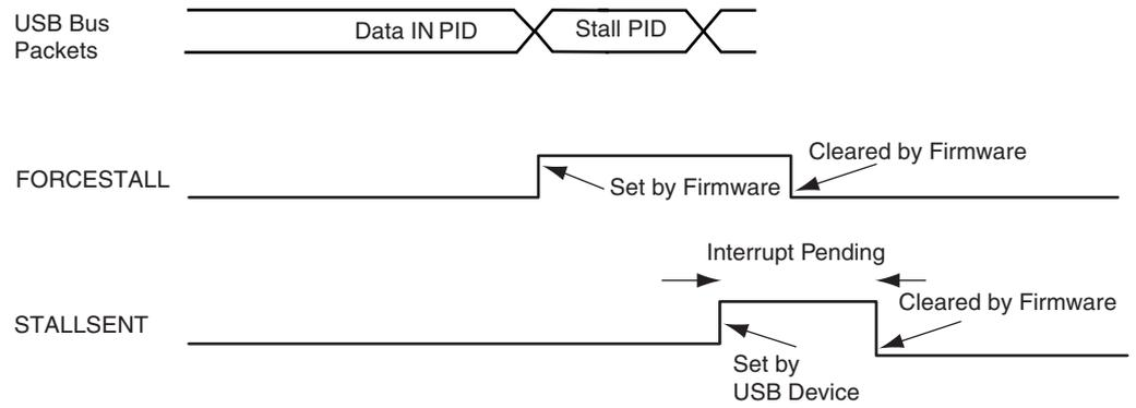
**Figure 117.** Stall Handshake (Data OUT Transfer)
