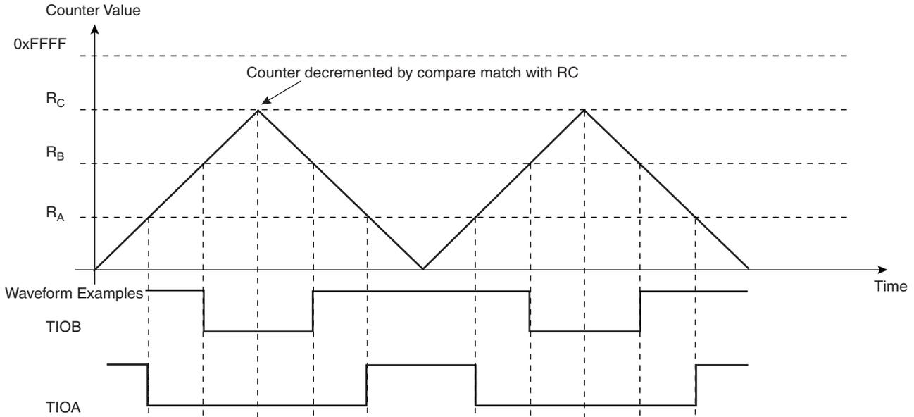
**Figure 97. WAVSEL = 11 With Trigger**
