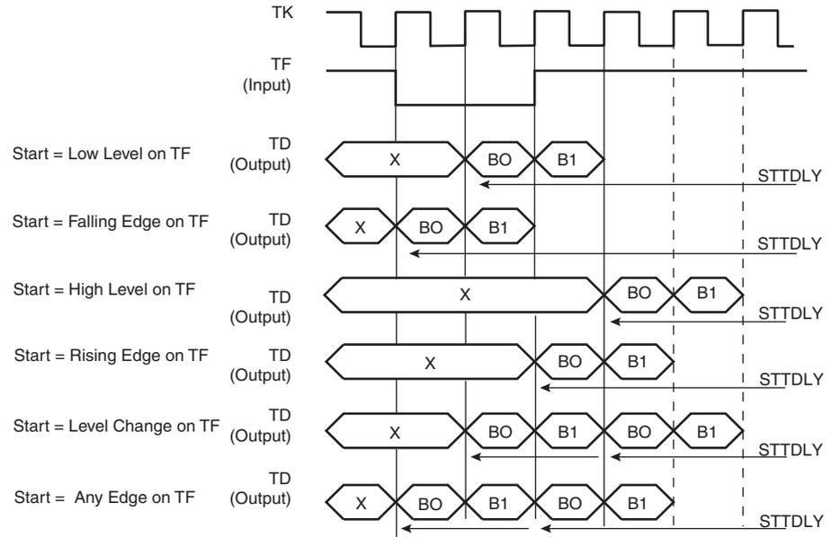
**Figure 77. Receive Pulse/Edge Start Modes**
