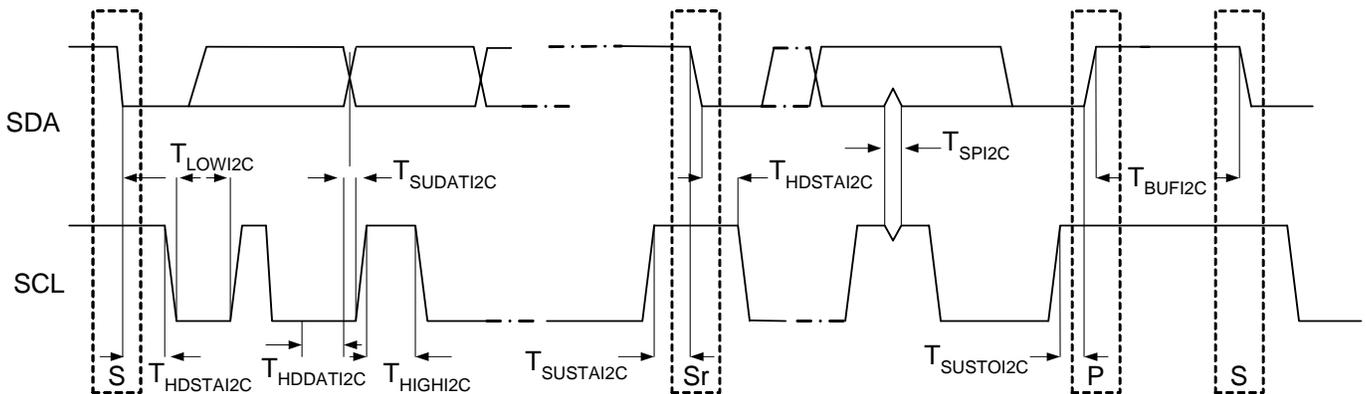
**Figure 3-9. Definition for Timing for Fast/Standard Mode on the I<sup>2</sup>C Bus**
