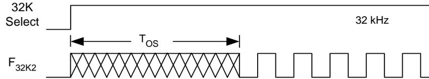
Figure 3-5. External Crystal Oscillator Startup Timing Diagram
