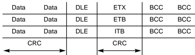
**Note:** For the transparent Bisync frames (receive only), the first DLE is not included in the CRC calculation, with the exception of DLE-SYN, in which the SYN is also not included.
