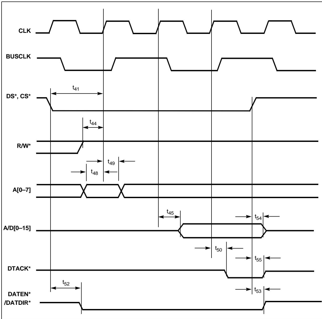
Figure 23. Slave Write Cycle Timing
