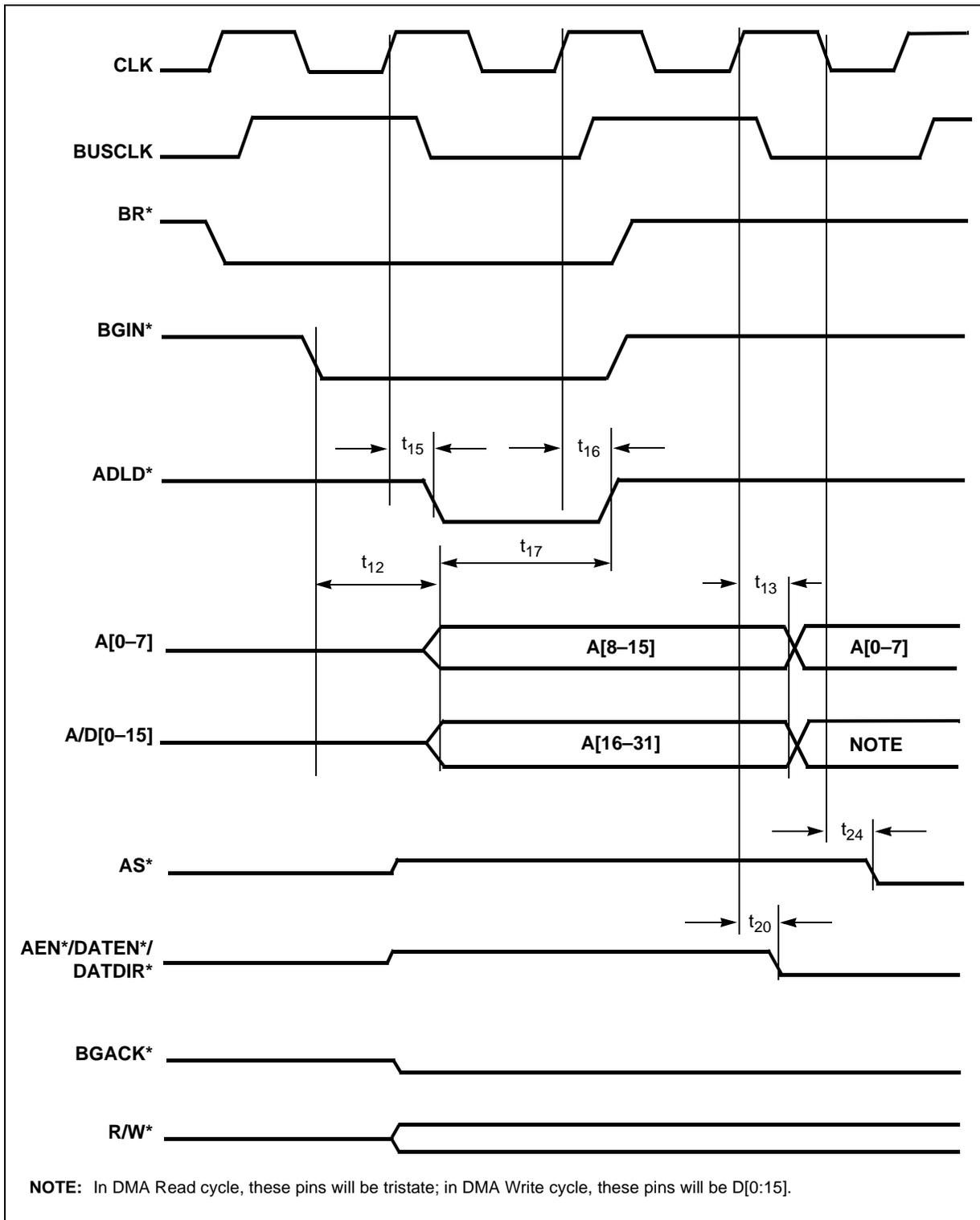
Figure 26. Bus Release Timing
