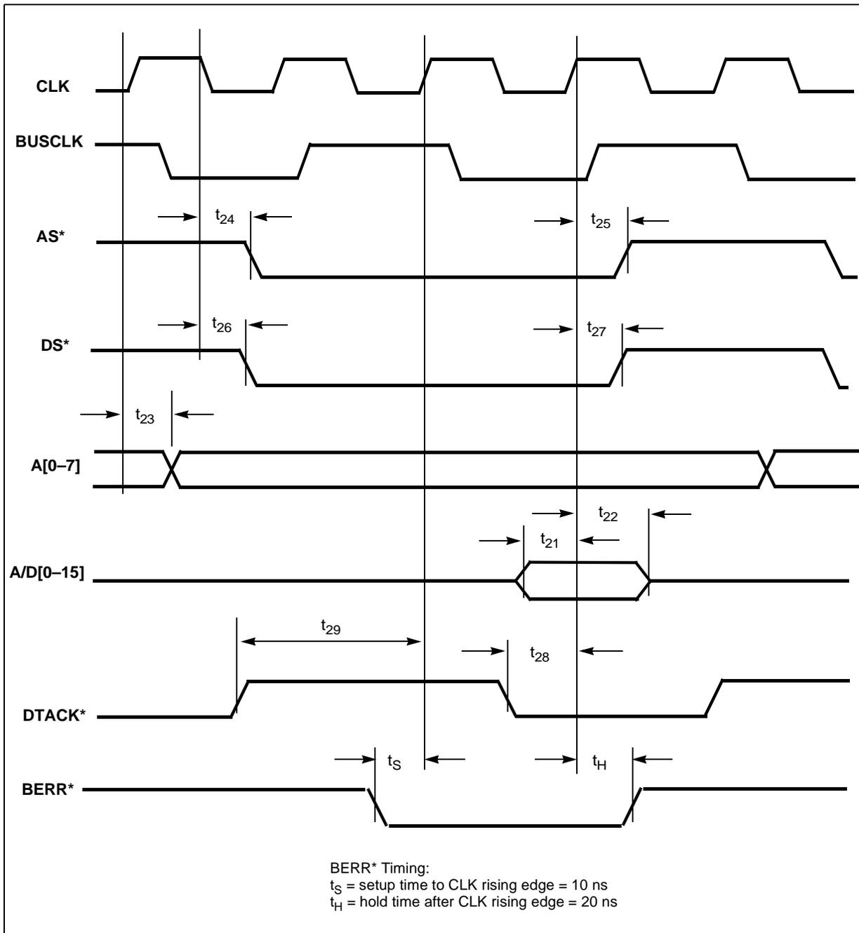
Figure 29. DMA Write Cycle Timing
