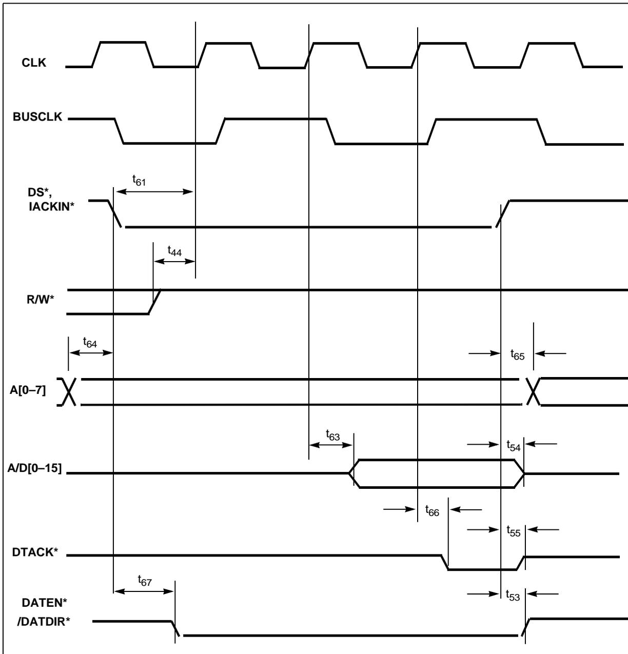
Figure 25. Bus Arbitration Cycle Timing
