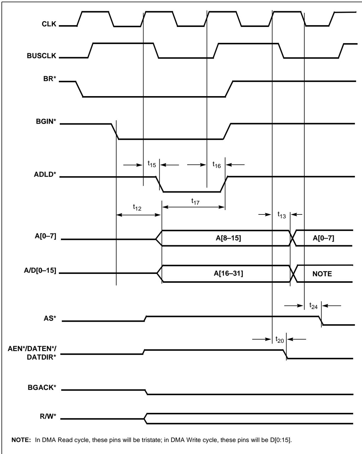
Figure 27. Bus Release Timing
