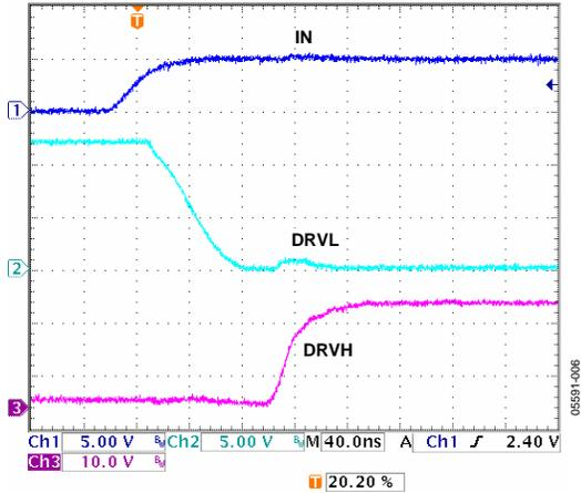
Figure 6. DRVH Rise and DRVL Fall Times
