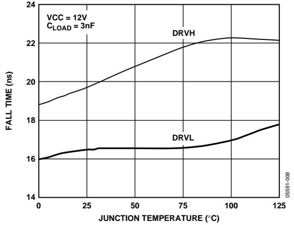
Figure 9. DRVH and DRVL Fall Times vs. Temperature
