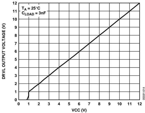
Figure 14. DRVL Output Voltage vs. Supply Voltage
