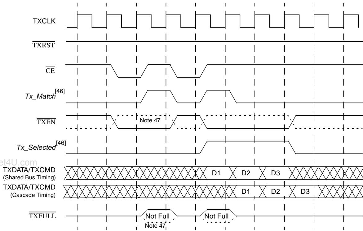
**Figure 8. Transmit Selection with Transmit FIFO Enabled**
