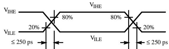
**CY7C9689 Transmitter TTL Switching Characteristics, FIFO Enabled Over the Operating Range**
