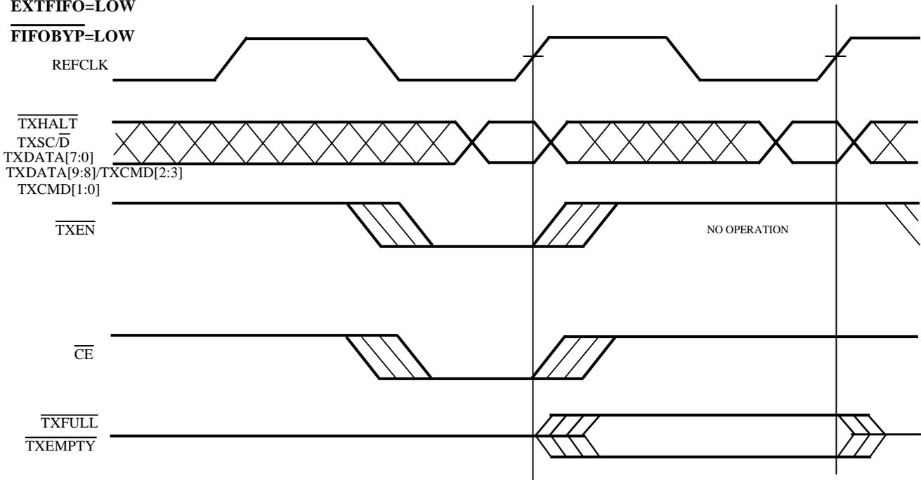
**CY7C9689 HOTLink Receiver Switching Waveforms**
