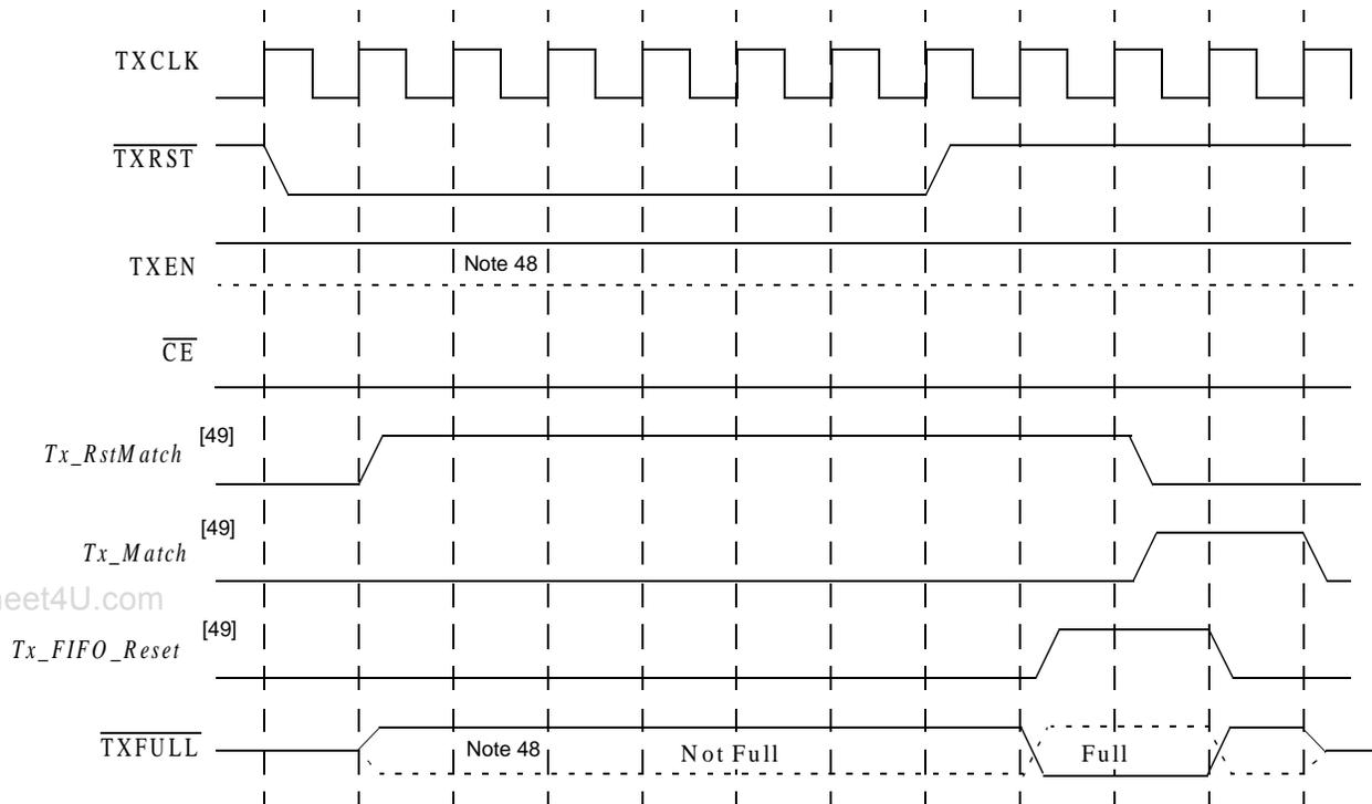
**Figure 14. Transmit FIFO Reset Sequence with Constant  $\overline{CE}$**
