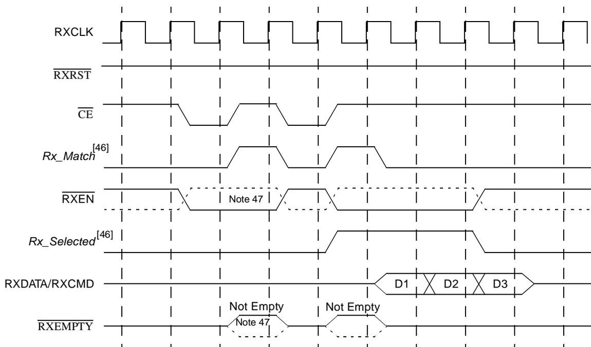
**Figure 10. Receive Selection with Receive FIFO Enabled**
