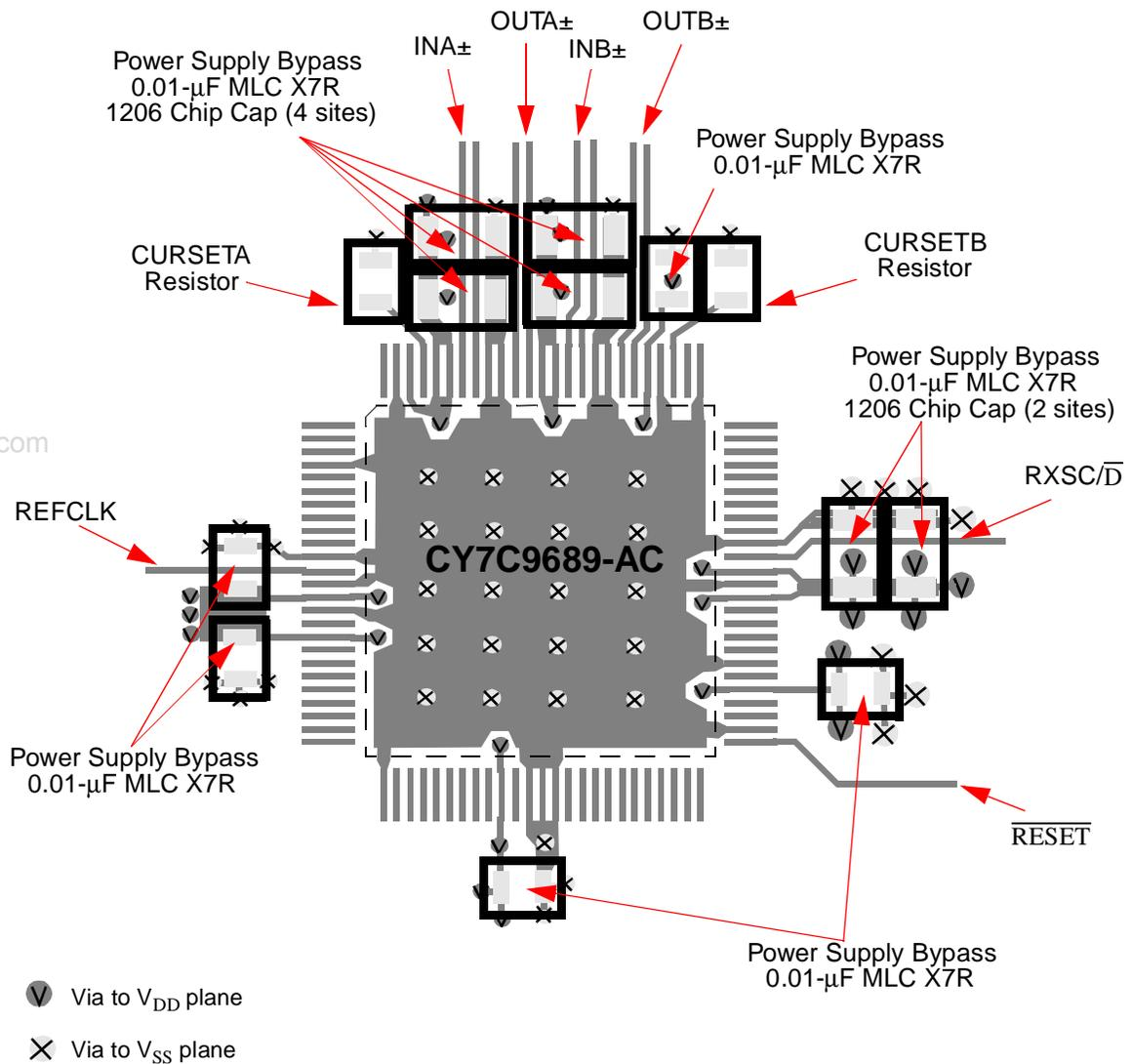
This is a typical printed circuit board layout showing example placement of power supply bypass components and other components mounted on the same side as the CY7C9689.
