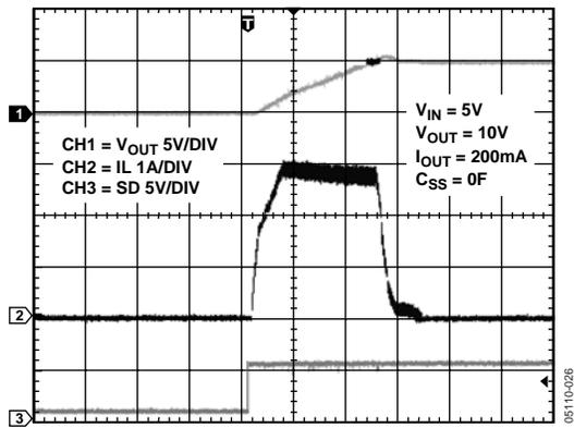
Figure 4. Start-Up Response from Shutdown,  $C_{SS} = 0F$
