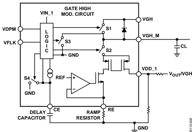
Figure 20. Gate Pulse Modulator Functional Block Diagram
