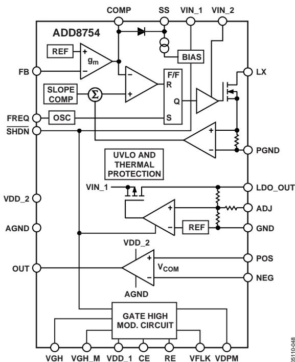
Figure 18. Detailed Functional Block Diagram
