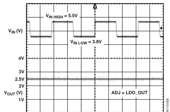
Figure 14. LDO Line Transient Response,  $V_{OUT} = 2.5\text{ V}$
