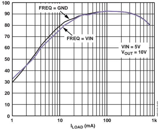
Figure 3. Efficiency vs. Load Current (mA)
