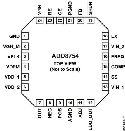
Figure 2. Pin Configuration
