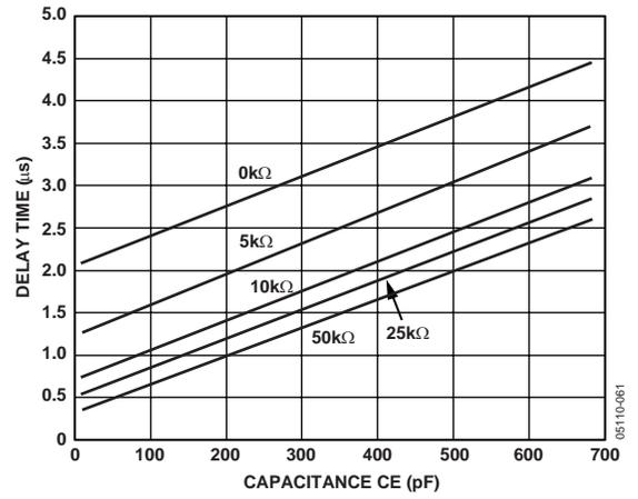
Figure 17. GPM Delay Time vs. CE Capacitance
