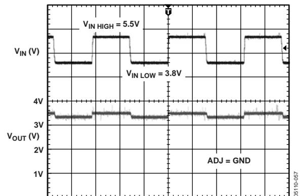
Figure 13. LDO Line Transient Response,  $V_{OUT} = 3.3\text{ V}$
