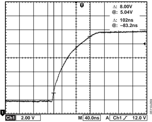
Figure 15.  $V_{COM}$  Rising Slew Rate,  $VDD_2 = 14V$
