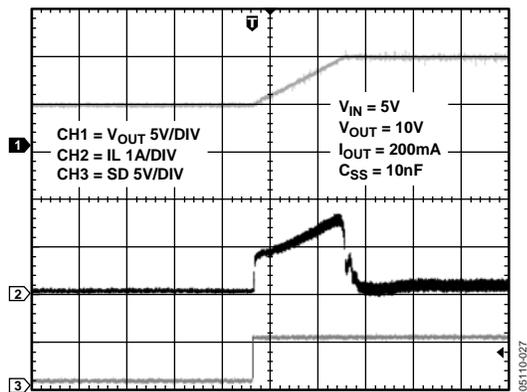
Figure 5. Start-Up Response from Shutdown,  $C_{SS} = 10F$
