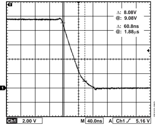
Figure 16.  $V_{COM}$  Falling Slew Rate,  $VDD_2 = 14V$
