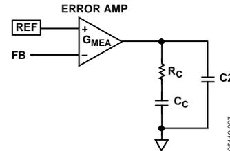
Figure 19. Compensation Components
