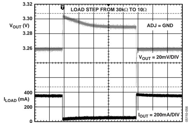
Figure 12. LDO Load Transient Response,  $V_{OUT} = 3.3\text{ V}$
