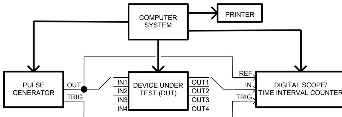
Figure 2: Test Setup
