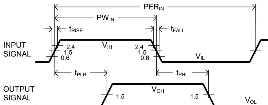
Figure 3: Timing Diagram
