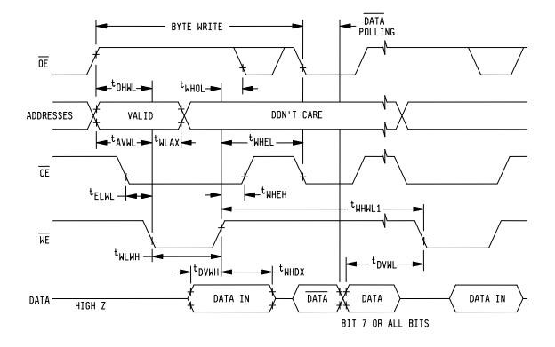
FIGURE 6. WE controlled byte write programming waveform.
