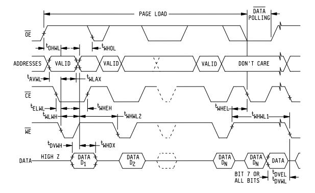
Note: The page write operation of the device allows 2 to 64 bytes of data to be loaded into the device and then simultaneously written during the internal programming period.
