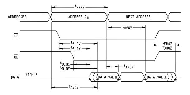
FIGURE 4. Timing waveforms.
