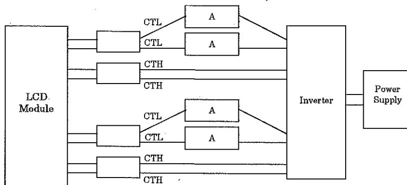
\*2) Lamp frequency of inverter may produce interference with horizontal synchronous frequency, and this may cause horizontal beat on the display. Therefore, please adjust lamp frequency, and keep inverter as far from module as possible or use electronic shielding between inverter and module to avoid the interference.
