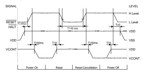
Please maintain the above sequence when turning on and off the power supply of the module.
