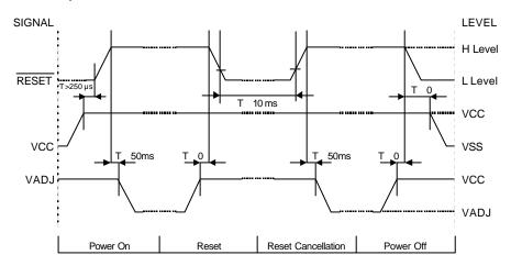
Please maintain the above sequence when turning on and off the power supply of the module. If VEE and/or VADJ is supplied to the module while internal alternate signal for LCD driving (M) is unstable or RESET is active, DC component will be supplied to the LCD panel. This may cause damage to the LCD module.
