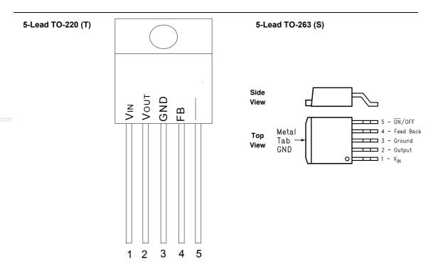
**+VIN** —This is the positive input supply for the IC switching regulator. A suitable input bypass capacitor must be present at this pin to minimize voltage transients and to supply the switching currents needed by the regulator.
