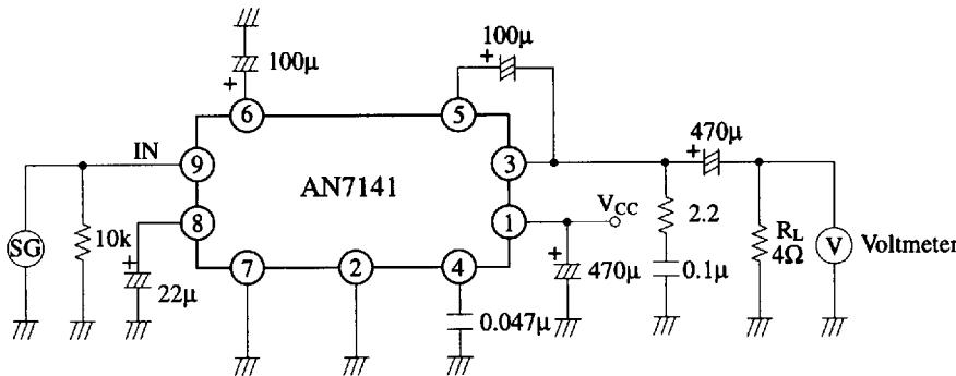
SG (Signal Generator) is separated from pin 9 at measurement of Quiescent Current and Output Noise Voltage.
